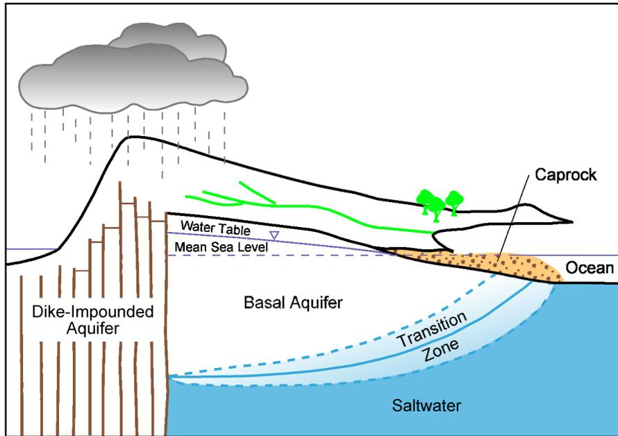
Figure 1. Hydrogeological features of a typical Hawaii basal aquifer
