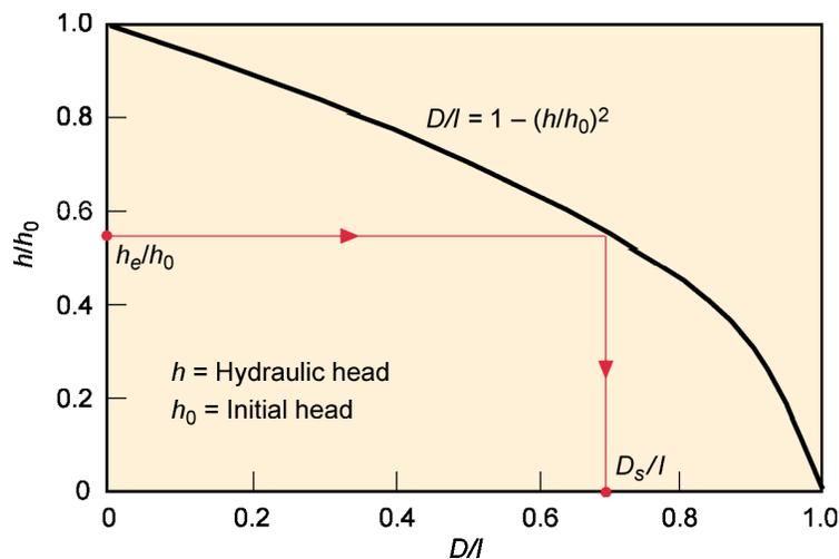
Figure 2. Basal aquifer head–draft curve derived by RAM to determine sustainable yield
