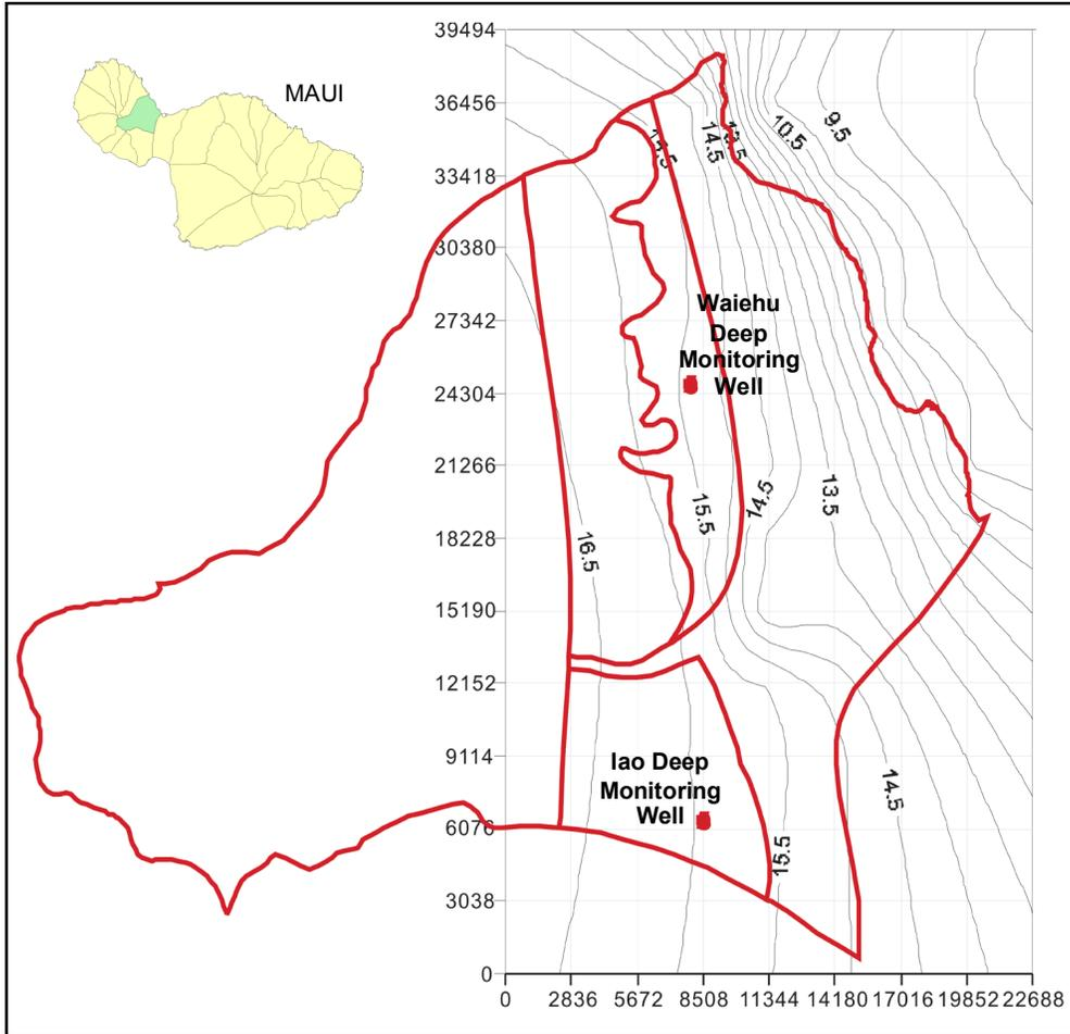
Figure 11. Hydraulic head contour of Iao aquifer, simulated by SHARP
