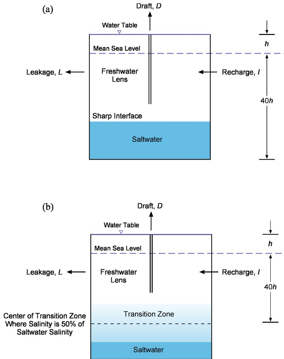
Figure 5. Conceptual formulation of (a) RAM as a CSTR with a sharp interface and (b) RAM2 as a CSTR with a transition zone
