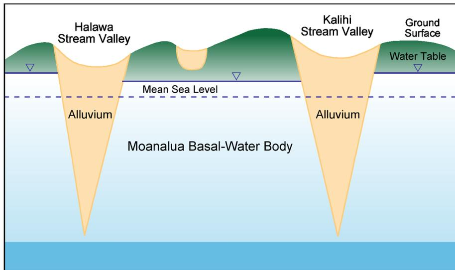
Figure 25. Geologic cross-section of Moanalua basal-water body in Honolulu aquifer
