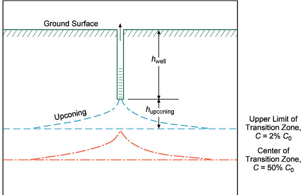
Figure 7. Upconing under a pumping well in a basal aquifer
