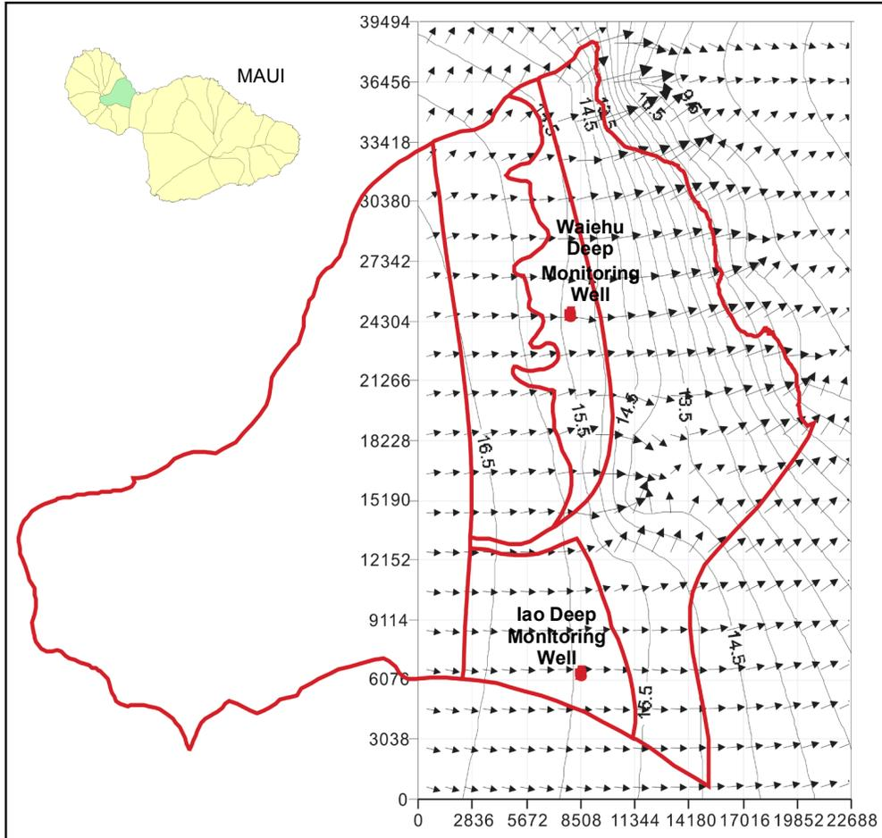
Figure 12. Groundwater flow net of Iao aquifer, simulated by SHARP
