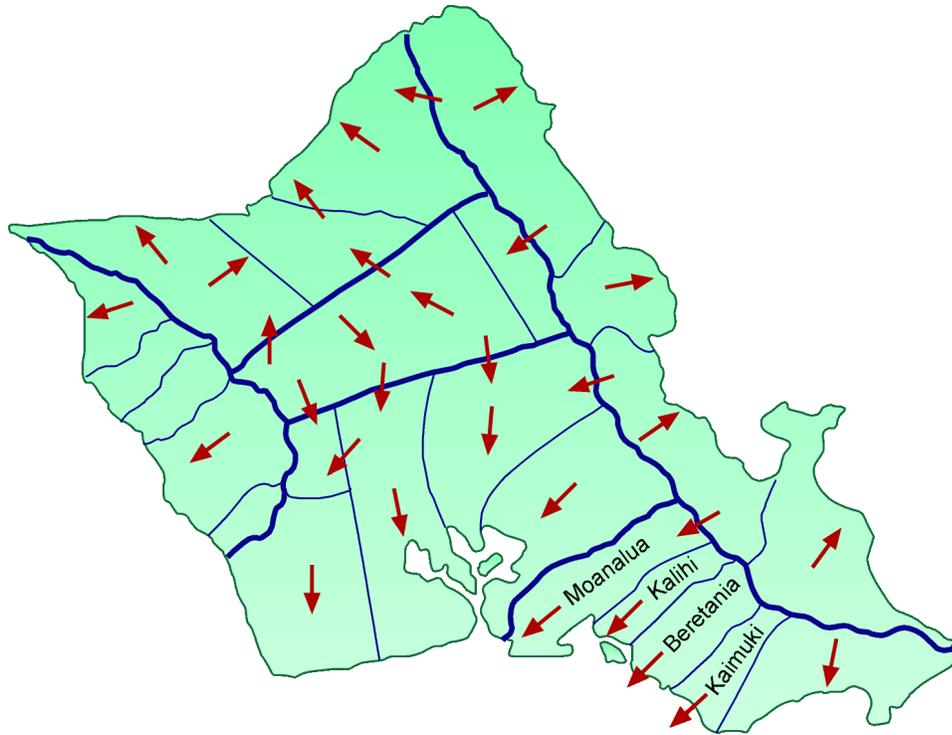
Figure 26. Water movement of Oahu aquifer systems (modified from Oki, 2005)
