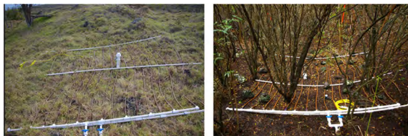
Figure 6. Photo of typical 2.5 × 2.5 m plots in the grassland and forest, showing irrigation tubing used for infiltration experiment.
