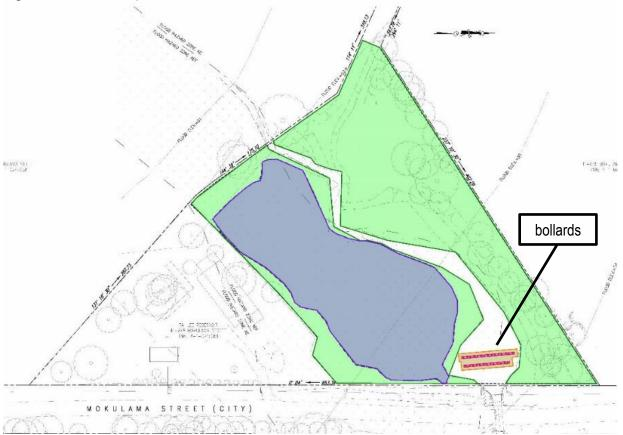
Each of the 28 steel bollards (8-inch diameter) will be provided with a six (6) foot depth by two (2) foot diameter cast-in-place concrete footing and will extend a maximum of four (4) feet above finish grade. The proposed grouted rip-rap area will cover an area of 956 square feet with a depth of two (2) feet for a volume of 1,912 cubic feet. The contractor may be required to use casing while installing the steel bollard concrete footings to prevent collapse of the drilled holes.
