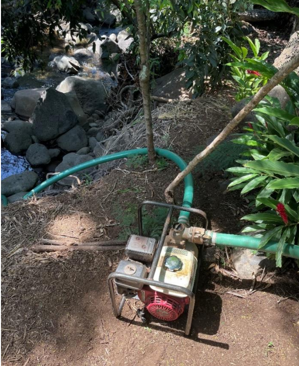
Site F: 2-inch hose attached to a 152 gpm pump on the right bank of Kahoma Stream.
