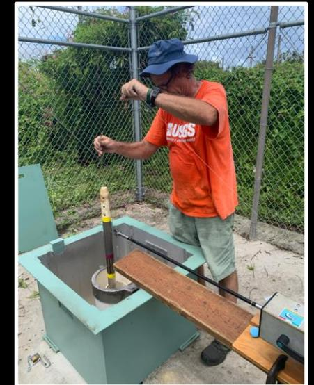
Conductivity, temperature and depth profiling at deep monitoring well EX-9, Guam
