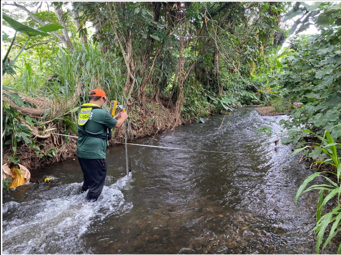
Hydrographer measuring discharge at Waiāhole Stream, O'ahu
