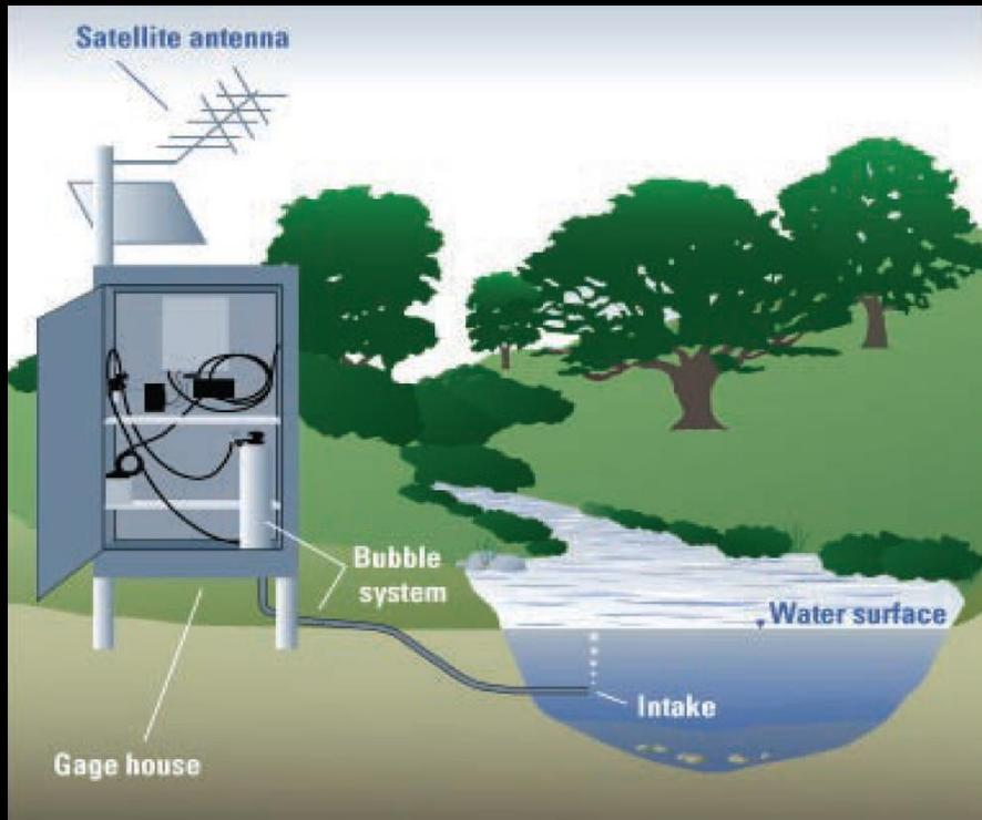
A stream gage measures and records the water level (called stage or gage height) of a stream or river.
