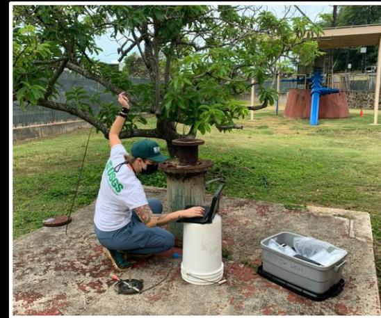
Groundwater-level measurement at Tripler Army Medical Center, O'ahu
