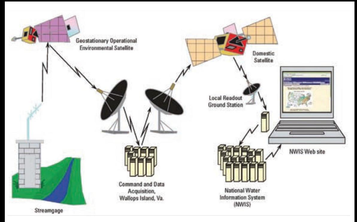
Data from the stream gage are transmitted via satellite to ground stations and relayed to USGS servers that host NWIS Web, a publicly accessible database.
