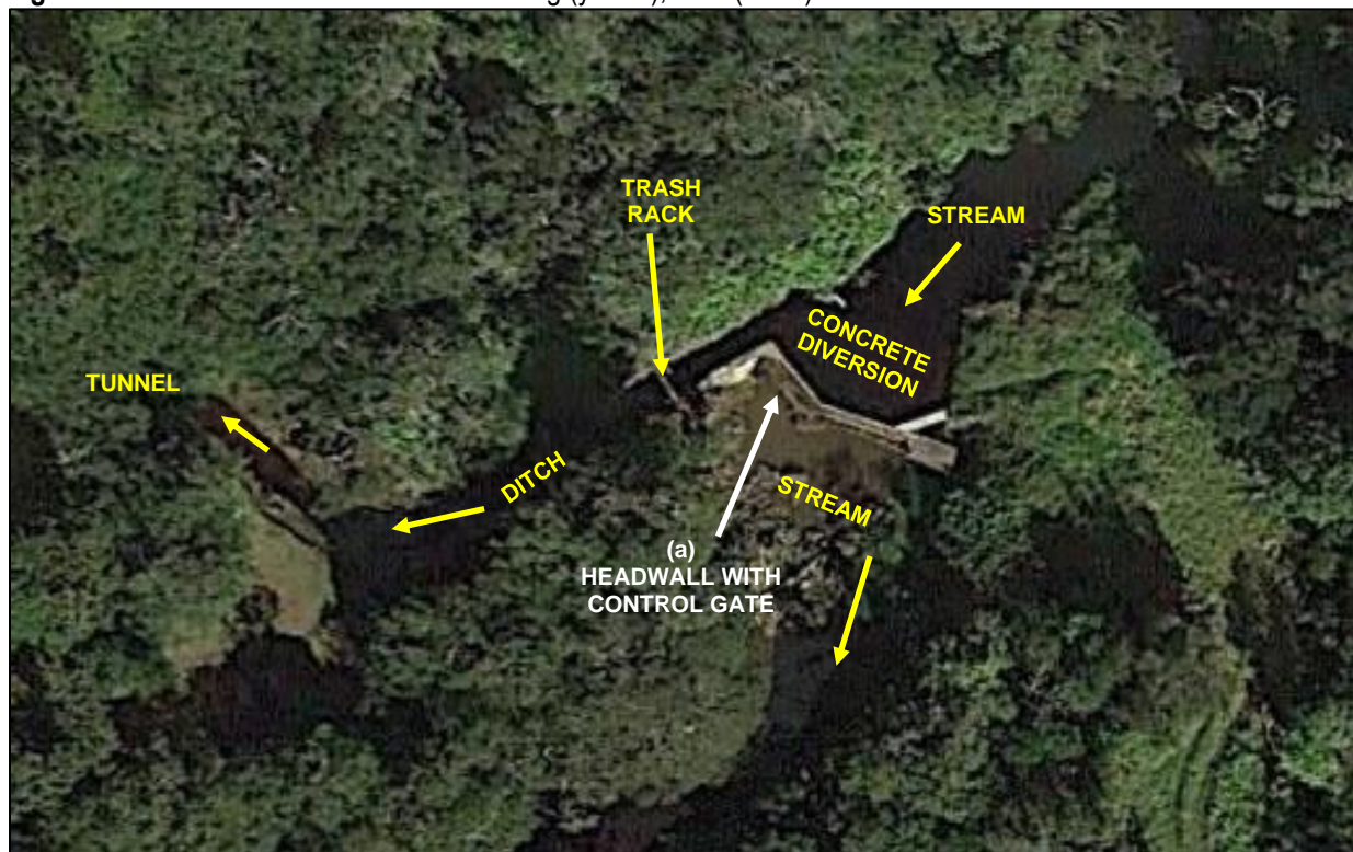
Figure 2. Waiakōali Stream Diversion. Existing (yellow), New (white).
