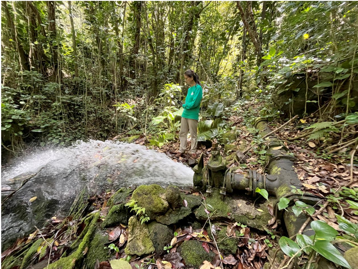
Figure 8. Discharge of approximately 300,000 gpd into Kaupuni Stream at approximately 1,400 ft. elevation.
