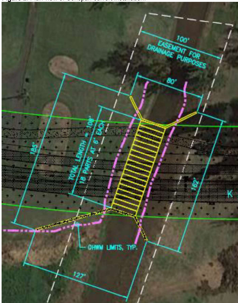
Figure 2: Plan view of Conspan culvert installation.
