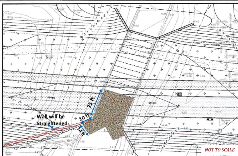
Plan View: Riprap Protection for CON/SPAN Culvert with Wingwalls
