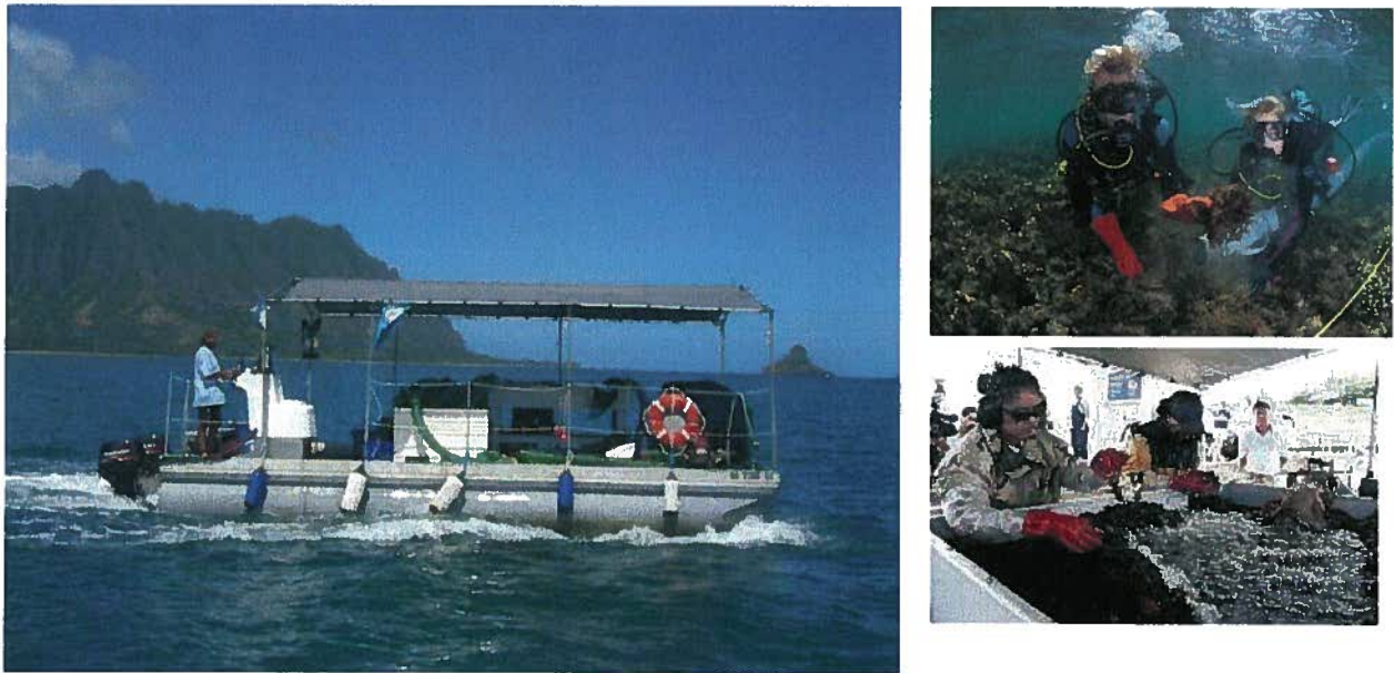
Figure 5. The Super Sucker is a Venturi type pump mounted on a barge with sorting table, dive compressor, and other equipment. Divers efficiently feed algae into a suction hose (top right). The algal material is deposited on the sorting table (bottom right) to remove native species. The algae are then bagged for transport to local farmers.
