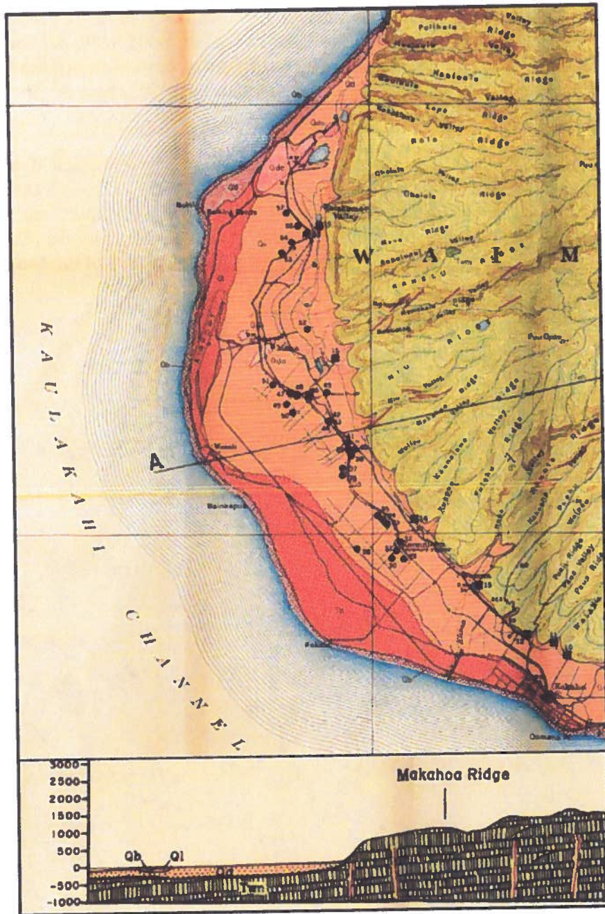
Figure 3.1 - 1. Regional geology of the Mānā Plain, island of Kauaʻi. Tw=nā Pali formation lava; Ql=Mānā Plain lagoon deposits; Qa=unconsolidated alluvium; Qd=calcareous sand dunes; Qb=beach sands; Qc=sand dune (from MacDonald et al. 1960).
