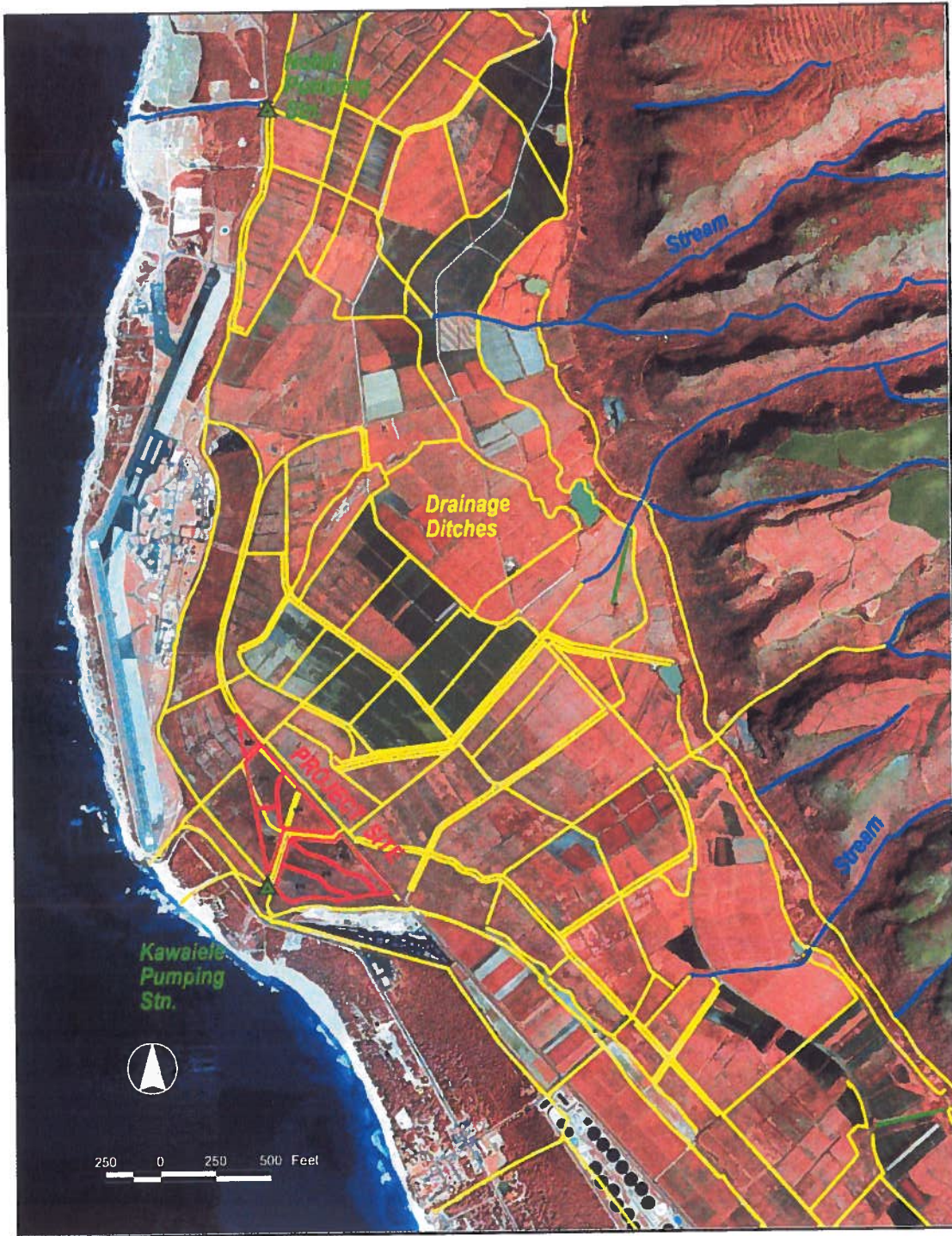
Figure 3.2 - 8. Local area surface water drainage system and pump stations on the Mānā Plain.
