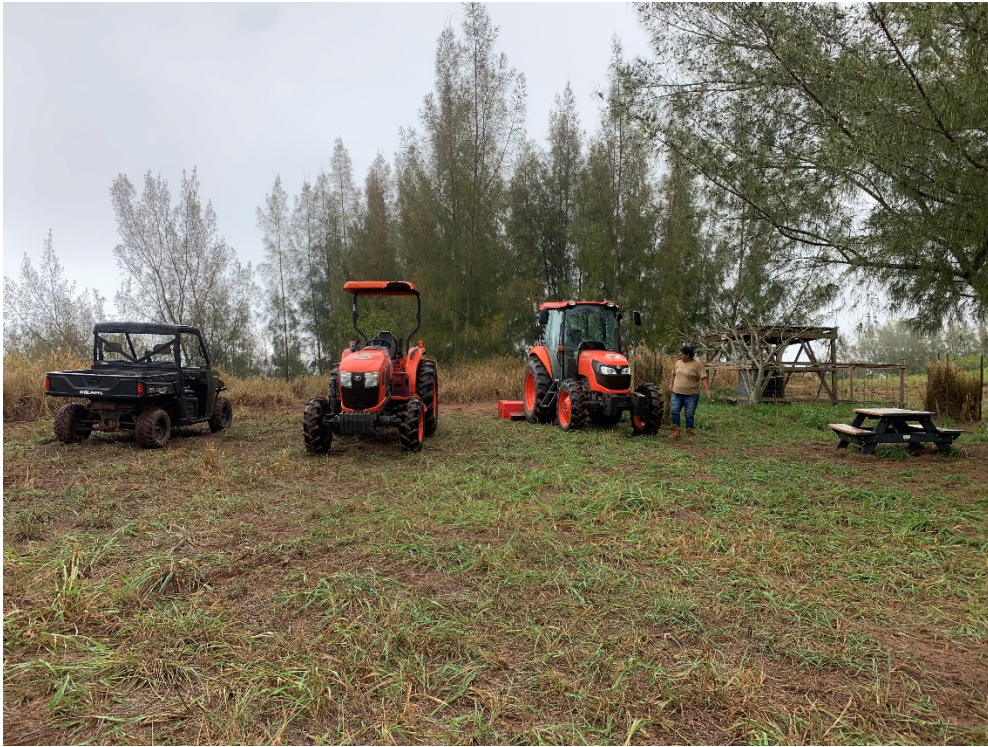
Figure 2. Starting from left to right, the Polaris Ranger, Kubota with rotary mower, Kubota with flail mower. This equipment is primarily used to help maintain all habitat and management areas for public hunting.
