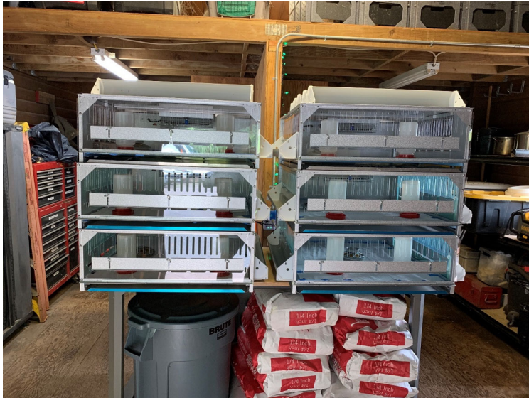
Figure 2-4. New Brooder Box Systems (GQF 0534 Universal Box Brooder). Nine were purchased to improve the rearing process of day-old chicks arriving on the island. Incorporated with self-regulating thermostats, outside feeders/waterers, and sliding soiled trays, it allows for much easier maintenance. The program will investigate obtaining more of these brooder systems since there was a higher survival rate using these compared to the aluminum troughs from last year. Troughs still prove helpful when the chicks pass four weeks of age.
