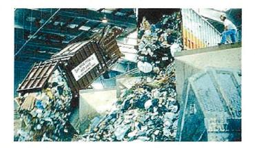
The facility's pre-processing system uses magnets to pull metals from the waste stream and eddy current separators extract non-ferrous metals from the ash, diverting approximately 18,000 tons of ferrous metals (e.g., tin cans) and 2,500 tons of non-ferrous metals (e.g., aluminum cans) to recycling annually. Moreover, H-POWER reduces our dependence on imported oil. One ton of trash produces saleable energy equivalent to 60 gallons of oil.
