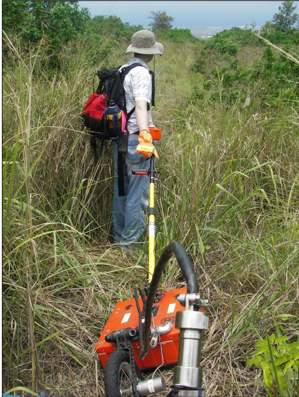
Plate 11. Escarpment Environmental technician Ian Moede pulls the ground penetrating radar (GPR) unit over the terrain at The Kula Nei Project area to assist with mapping of lava tubes.
