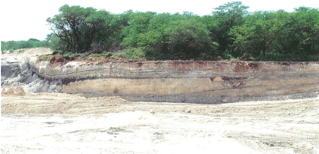
Figure 2. Pacific Aggregate (Mā'ili) Limestone Quarry. Quarry operations are mining an ancient limestone (reef) deposit, slowly removing the kiawe forest (background) on the northwest end of the property.
