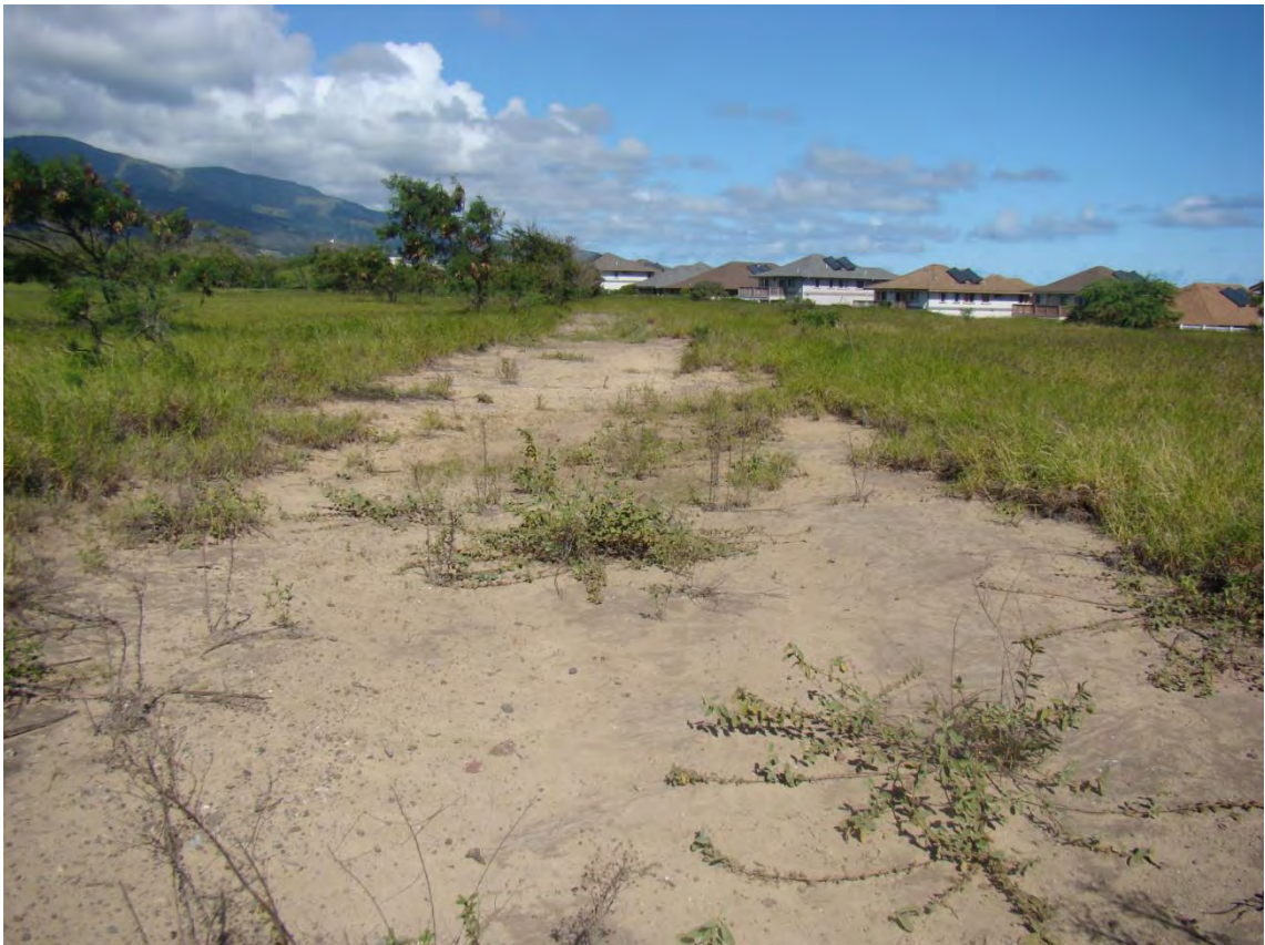
Sampling Area 1 – Open plain with loose sand and some exposed lithified sand at surface
