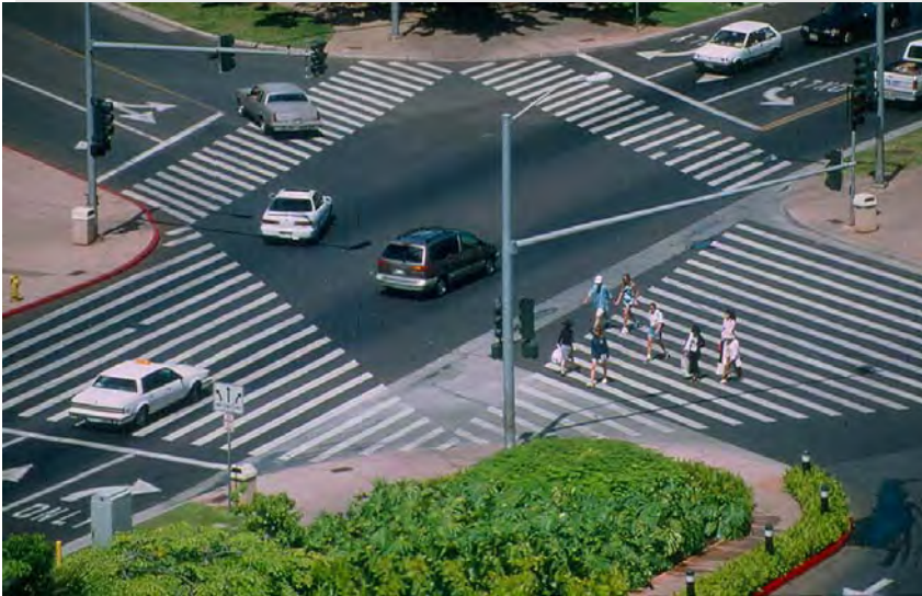
A Zebra Crossing is shown at the intersection of Kalia and Maluhia (left). Examples in Renton, Washington (below, left) and London (below, right) include “ Belisha Beacons ” poles with flashing lights triggered when the crosswalk is occupied.
