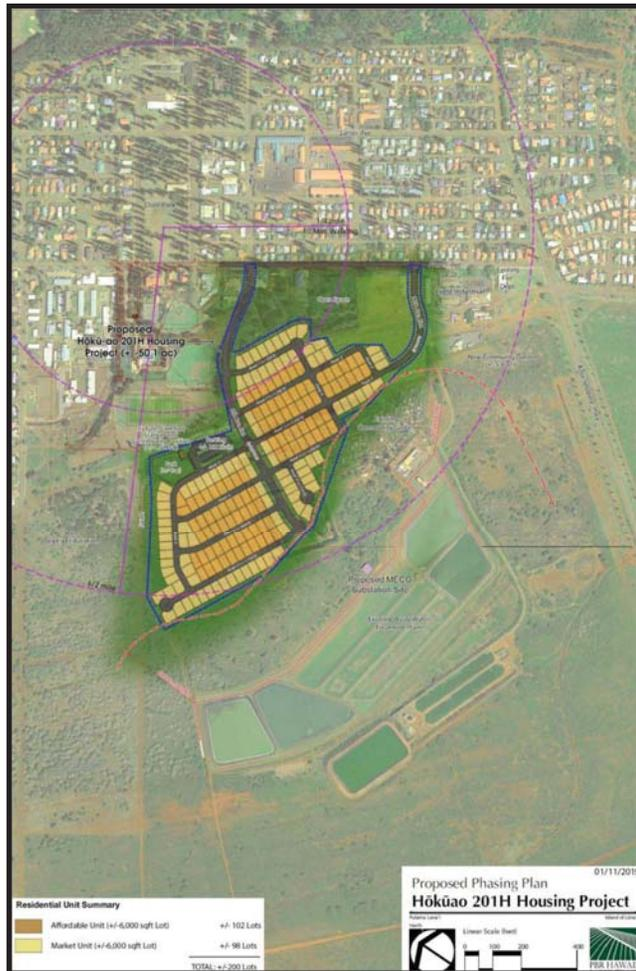
Figure 10. Conceptual site plan for the Hōkūāo 201-H housing project (Provided by Pūlama Lāna‘i)
