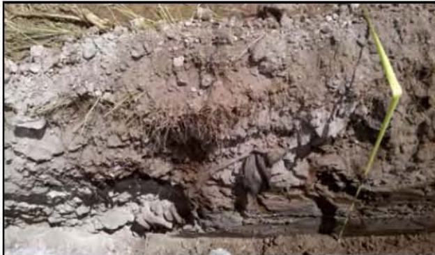
Figure 41. Test Trench 4, north wall, east end (note construction fabric in cross-cut trench).
