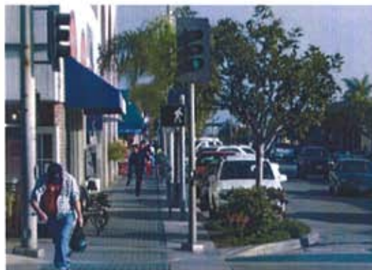
Traffic-calming device (bulb-out)
