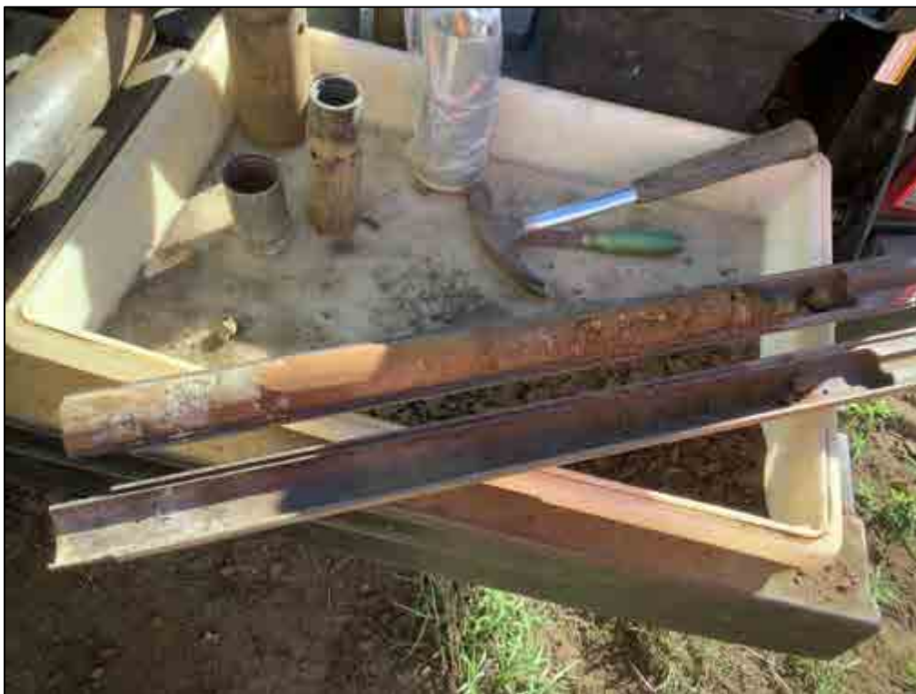
Figure 87. B-10, Sample 6 (5.5-6.0 m), gravel and fine silt
