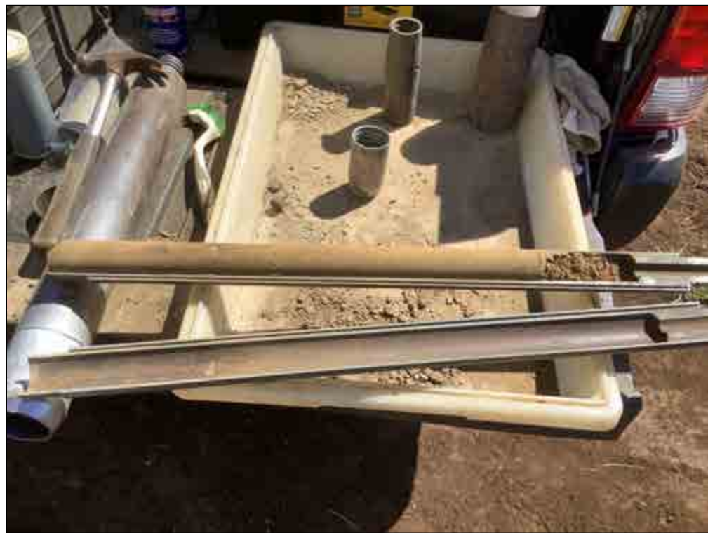
Figure 140. B-37, Sample 5 (4.1-4.5 m), sand
