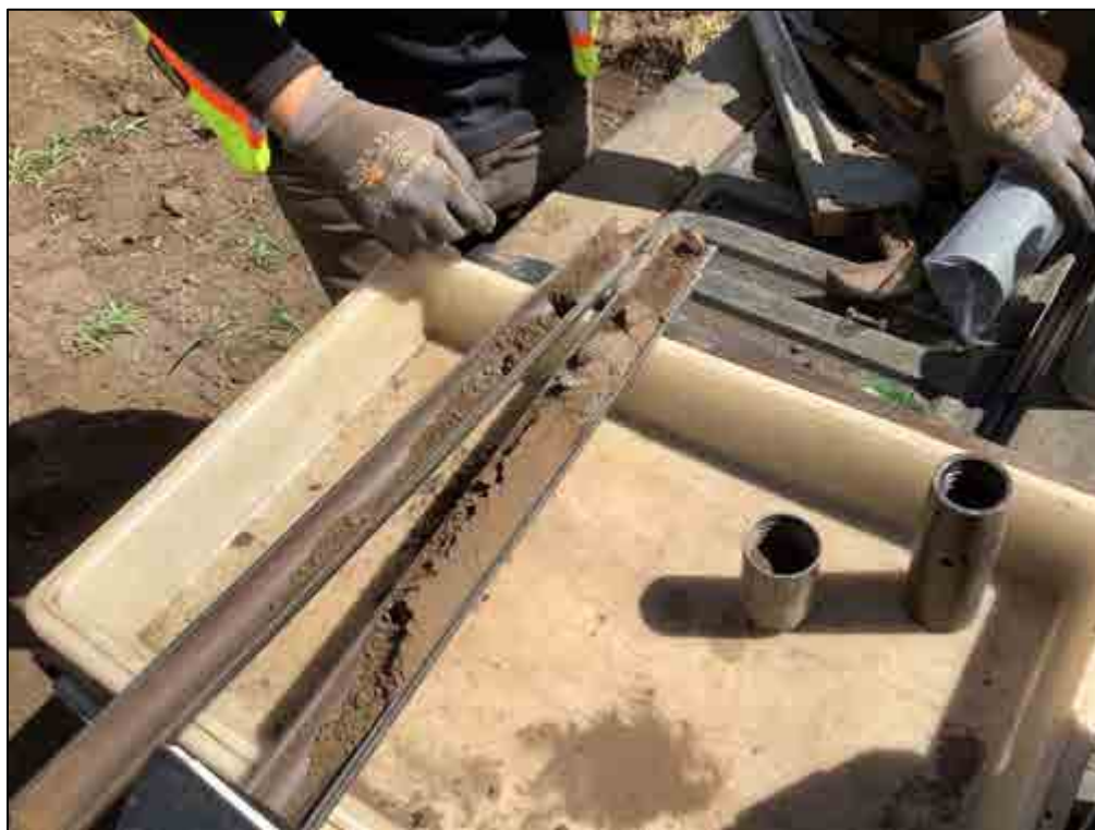
Figure 103. B-18, Sample 5 (4.1-4.5 m), silt loam and gravels
