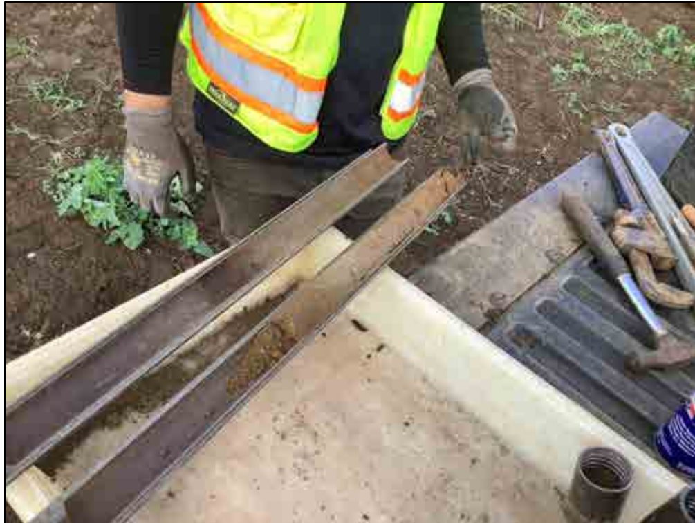
Figure 106. B-20, Sample 3 (1.5-1.9 m), sandy loam and silt loam
