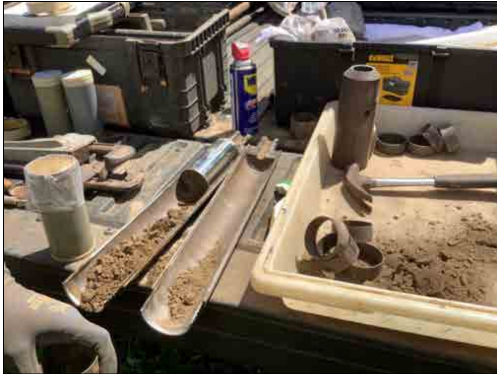
Figure 141. B-38, Sample 3 (1.5-1.9 m), loamy sand
