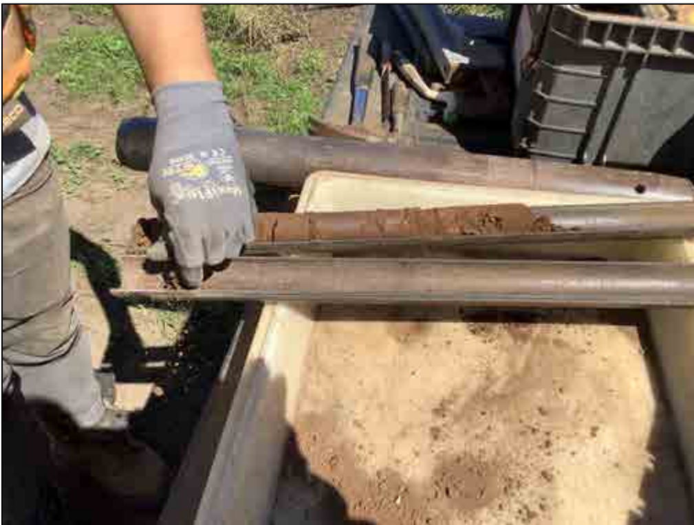
Figure 128. B-31, Sample 6 (5.5-6.0 m), silty clay loam
