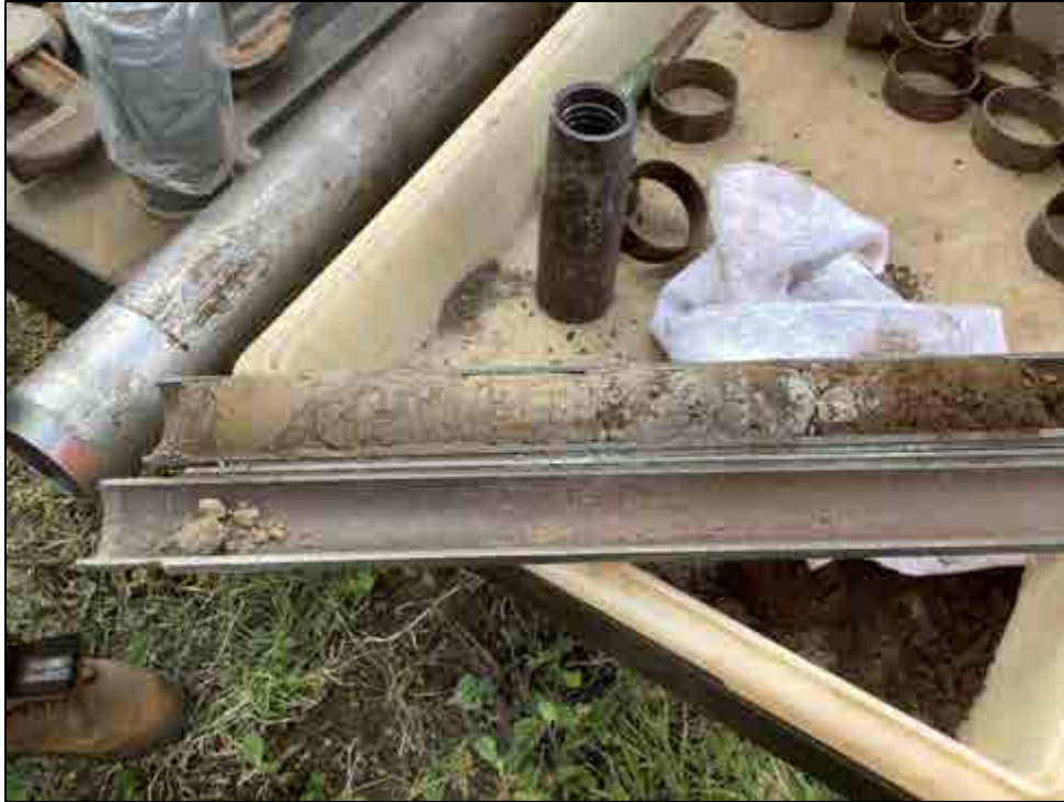
Figure 70. B-2, Sample 3 (1.5-1.9 m), sandy clay loam, loamy sand, and silt loam
