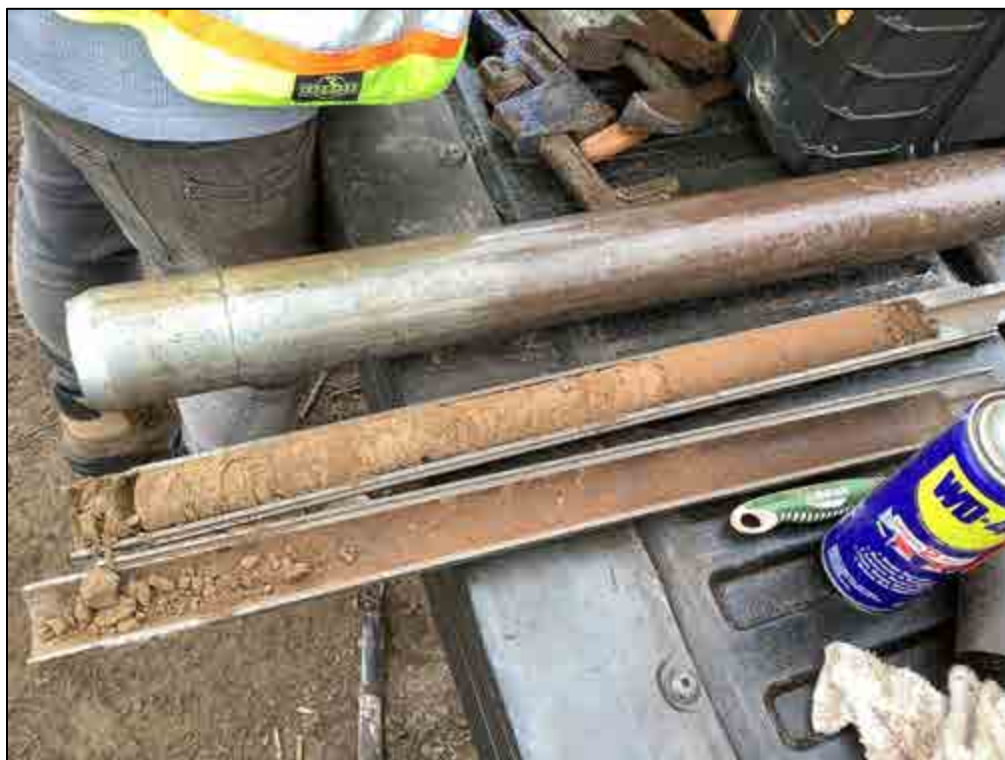
Figure 116. B-25, Sample 5 (4.1-4.5 m), silt loam
