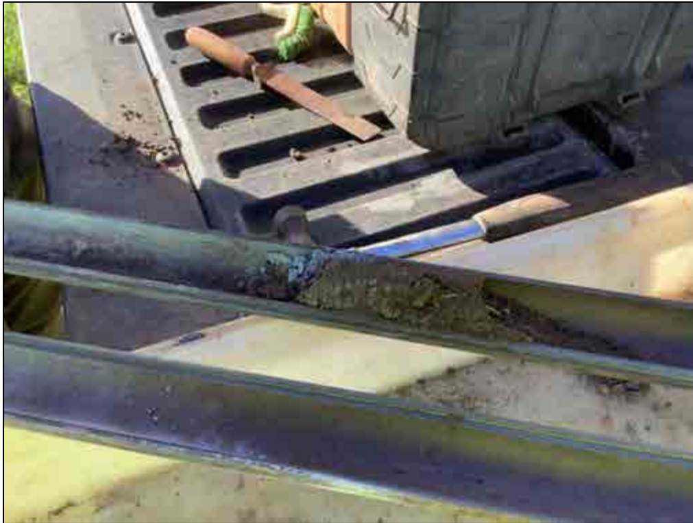
Figure 129. B-32, Sample 3 (1.5-1.9 m), sandy loam and alluvial deposited gravels
