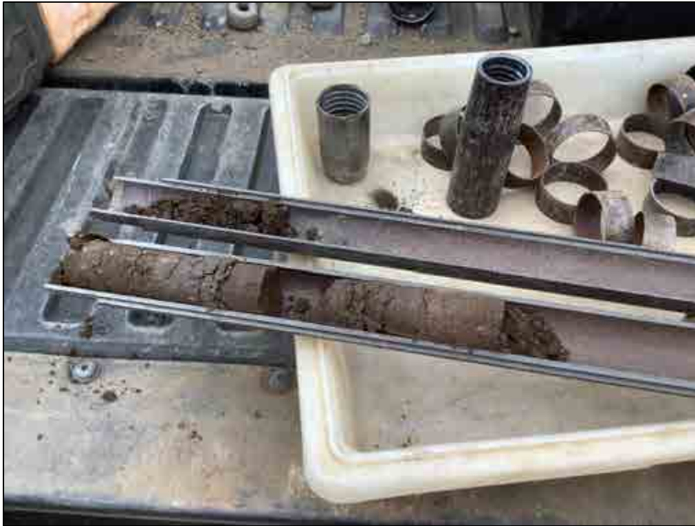
Figure 76. B-5, Sample 1 (0.4-0.9 m), sandy loam and sandy clay loam
