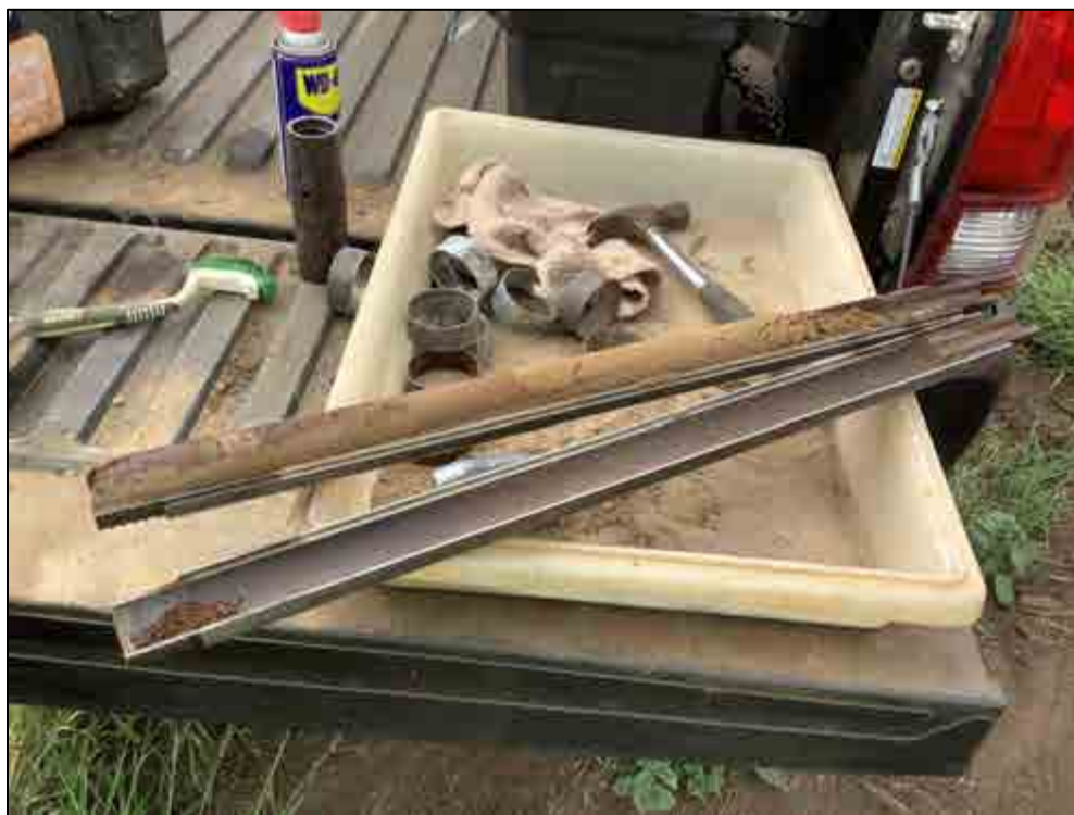
Figure 89. B-11, Sample 4 (2.5-3.0 m), sand and loamy sand
