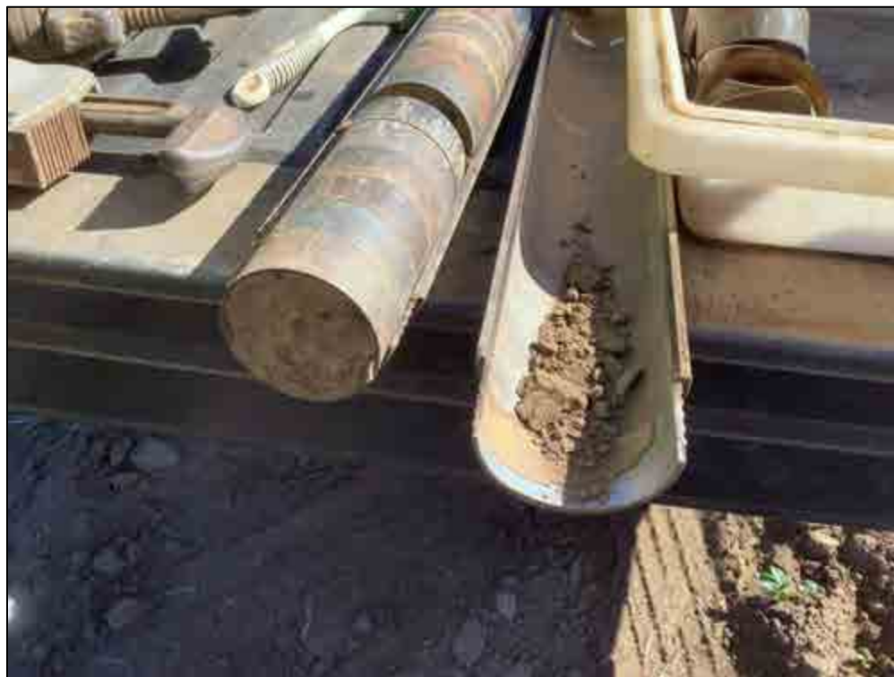
Figure 79. B-6, Sample 3 (1.5-1.9 m), silt loam
