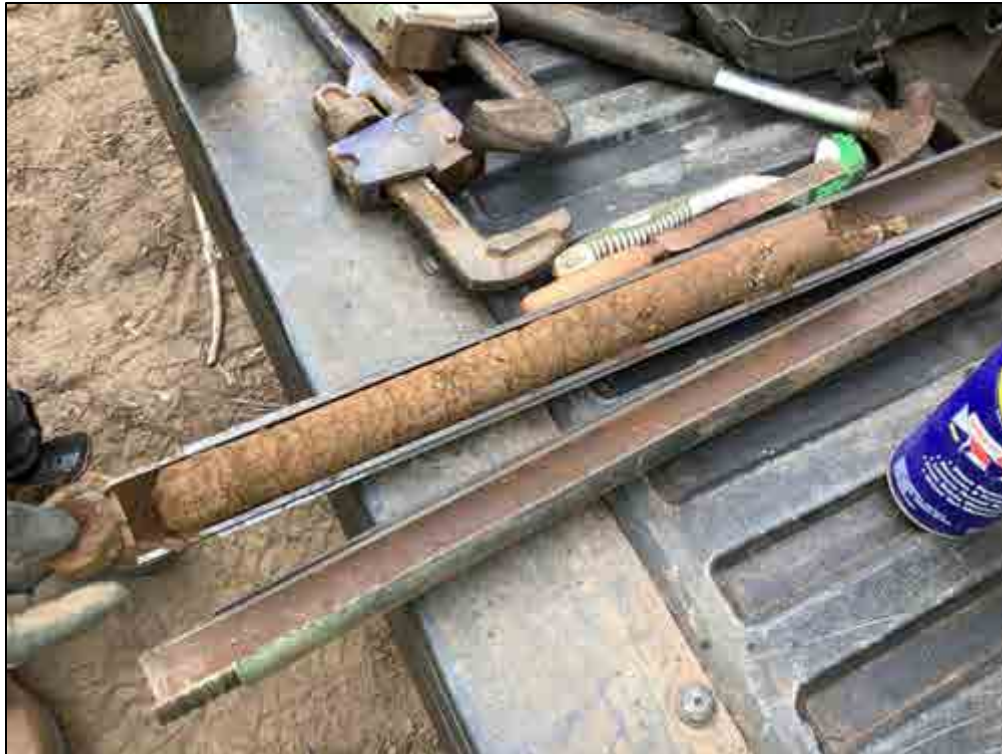
Figure 115. B-25, Sample 3 (2.5-3 m), silt loam and gravels
