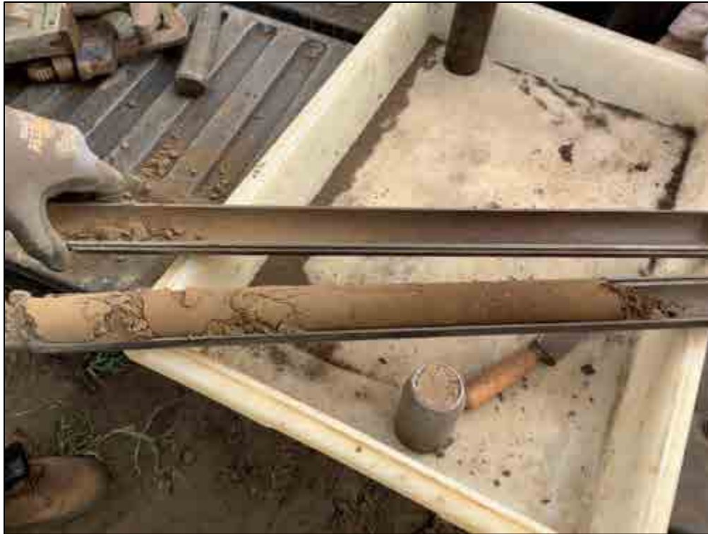
Figure 113. B-24, Sample 3 (1.5-1.9 m), silt loam
