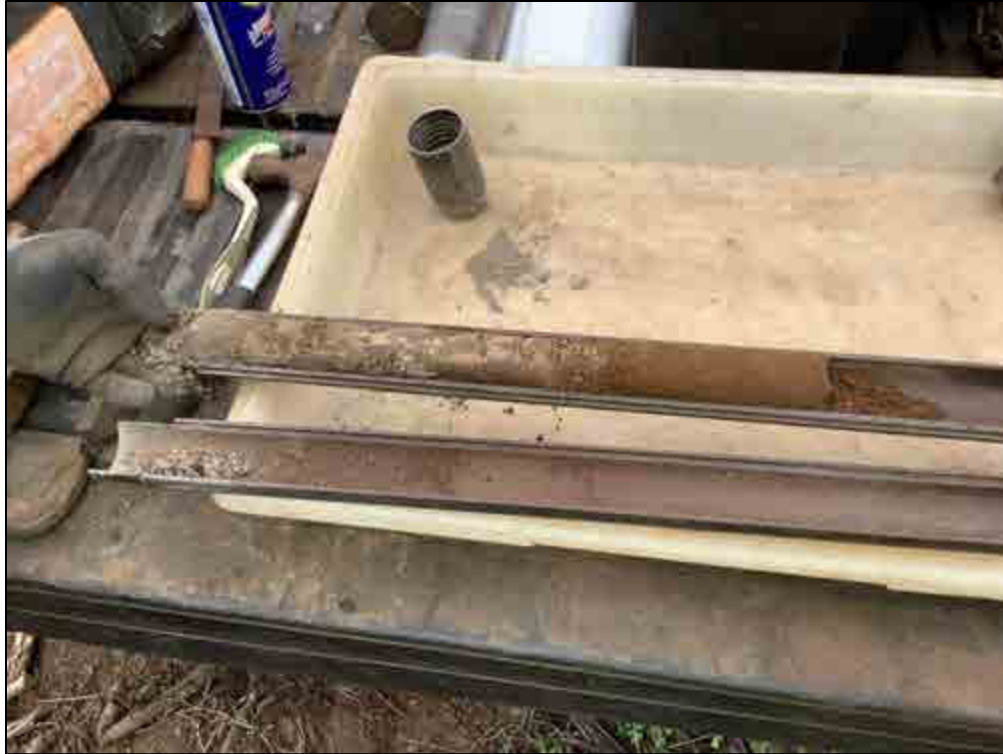
Figure 112. B-23, Sample 6 (5.5-6 m), silt loam and loamy sand with gravels
