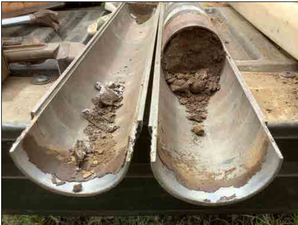
Figure 69. B-1, Sample 6 (5.5-6.0 m), sandy loam and gravels
