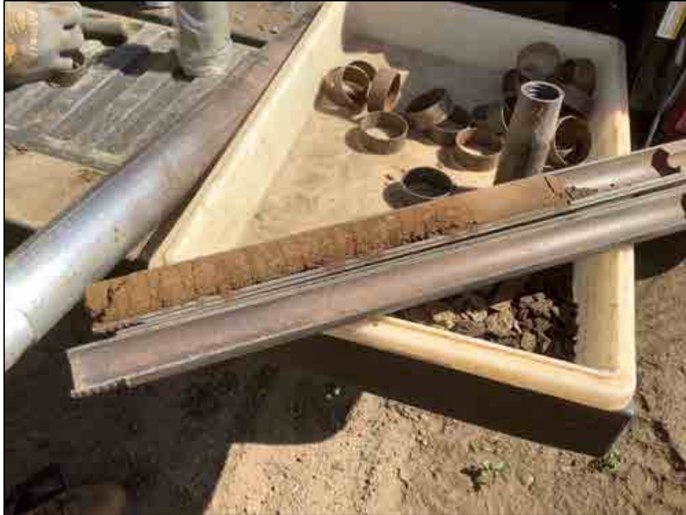
Figure 74. B-4, Sample 3 (1.5-1.9), silt loam
