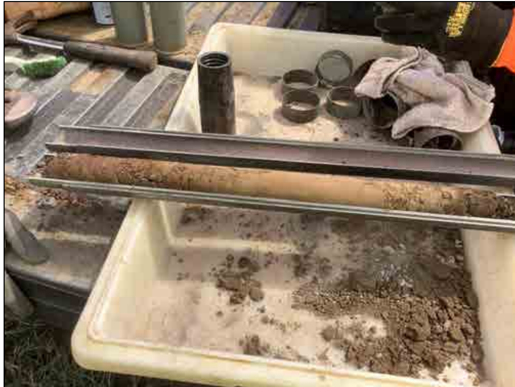
Figure 82. B-8, Sample 3 (1.5-1.9 m), silt loam
