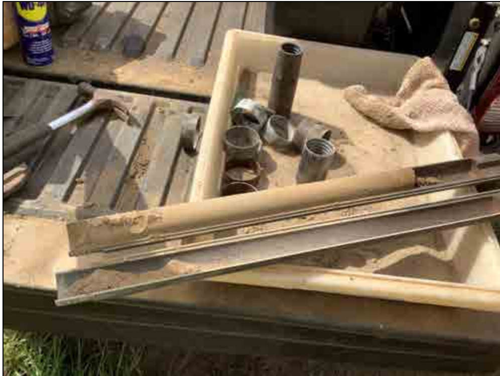
Figure 88. B-11, Sample 3 (1.5-1.9 m), sand and silt loam
