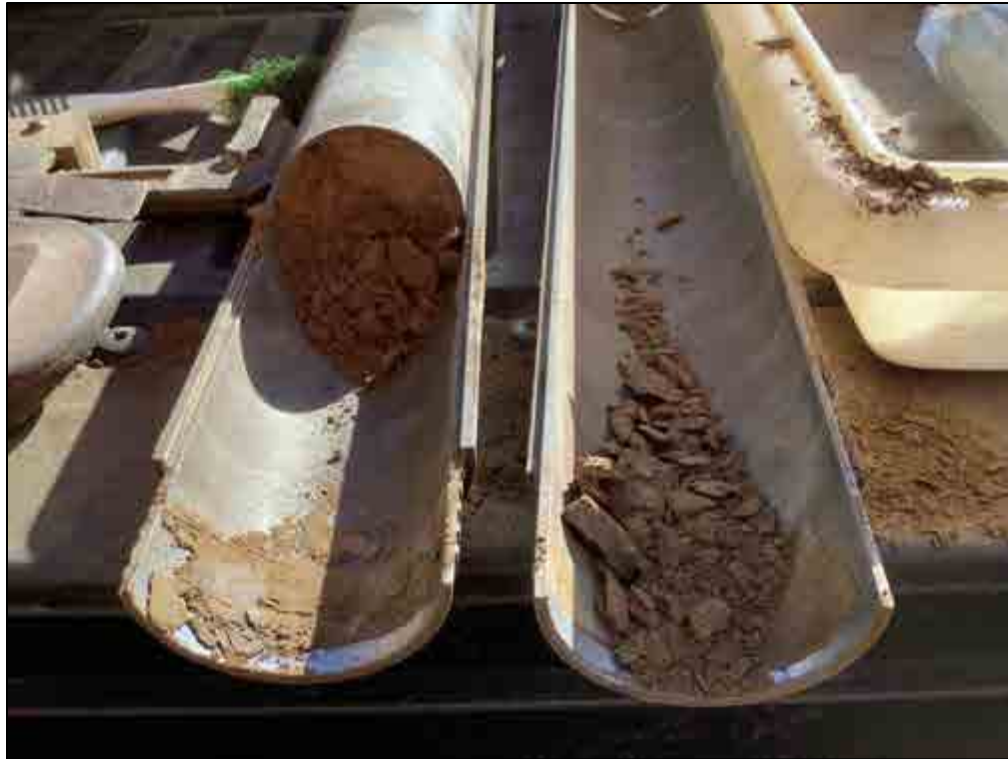
Figure 86. B-10, Sample 4 (2.5-3.0 m), silt loam
