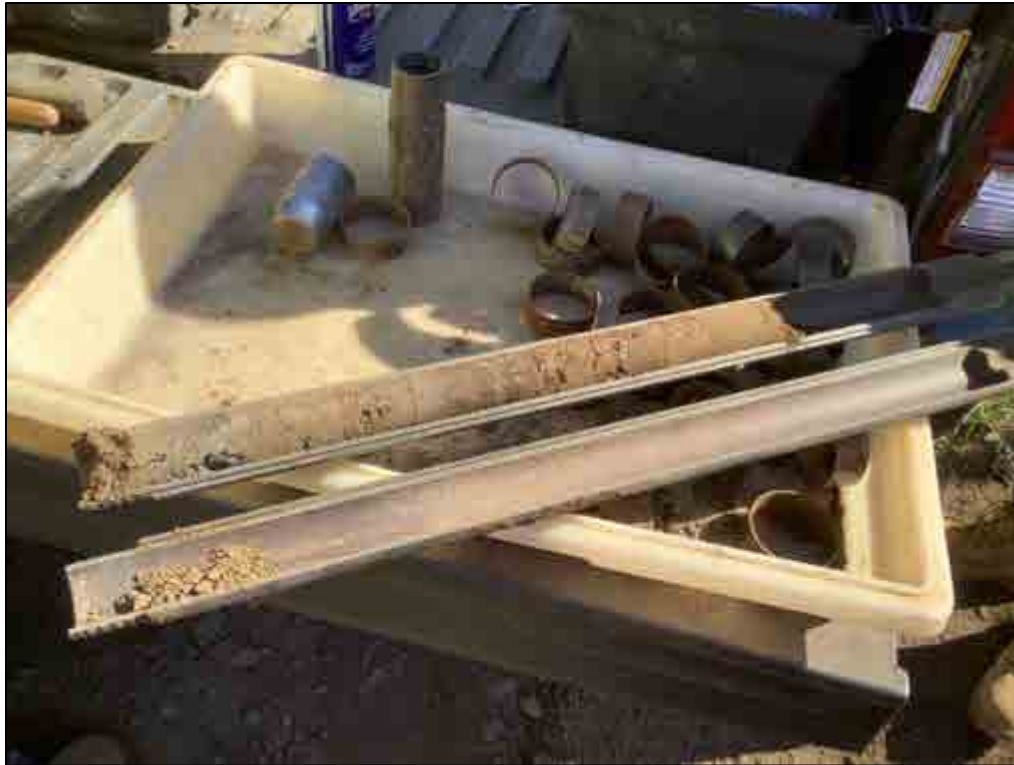
Figure 80. B-7, Sample 2 (0.9-1.5 m), silt loam
