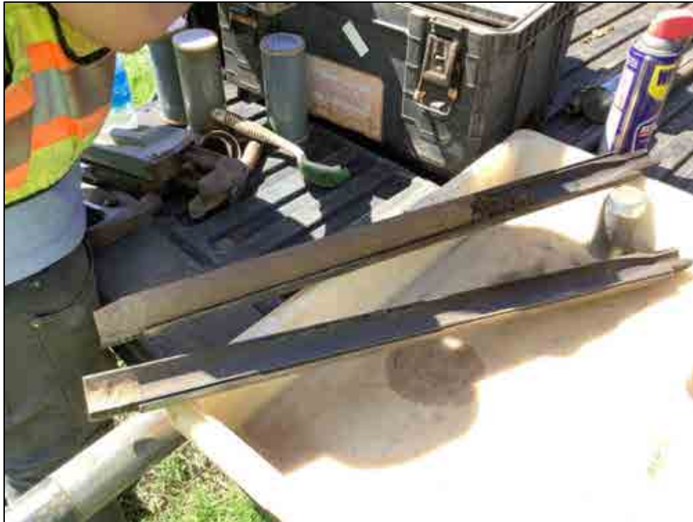
Figure 121. B-28, Sample 3 (1.5-1.9 m), sandy loam and loamy sand
