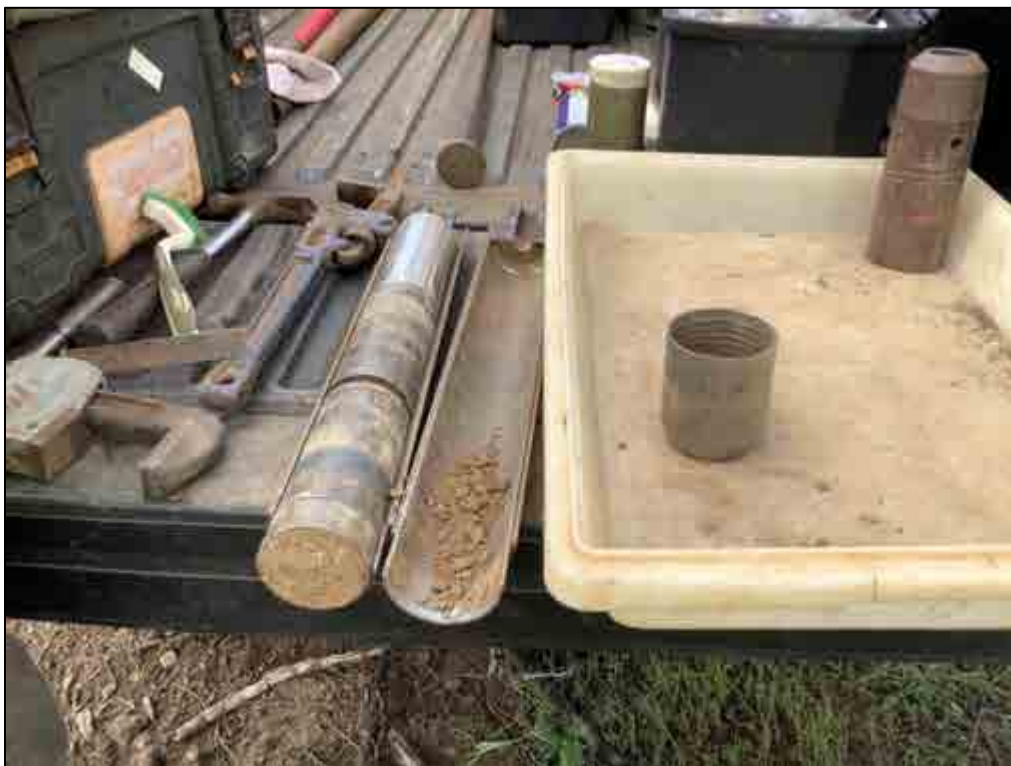
Figure 111. B-23, Sample 3 (1.5-1.9 m), silt loam
