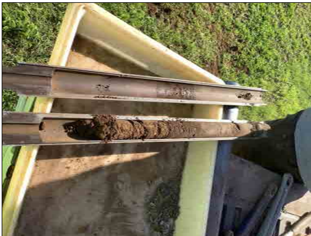
Figure 130. B-32, Sample 5 (4.1-4.5 m), silt loam
