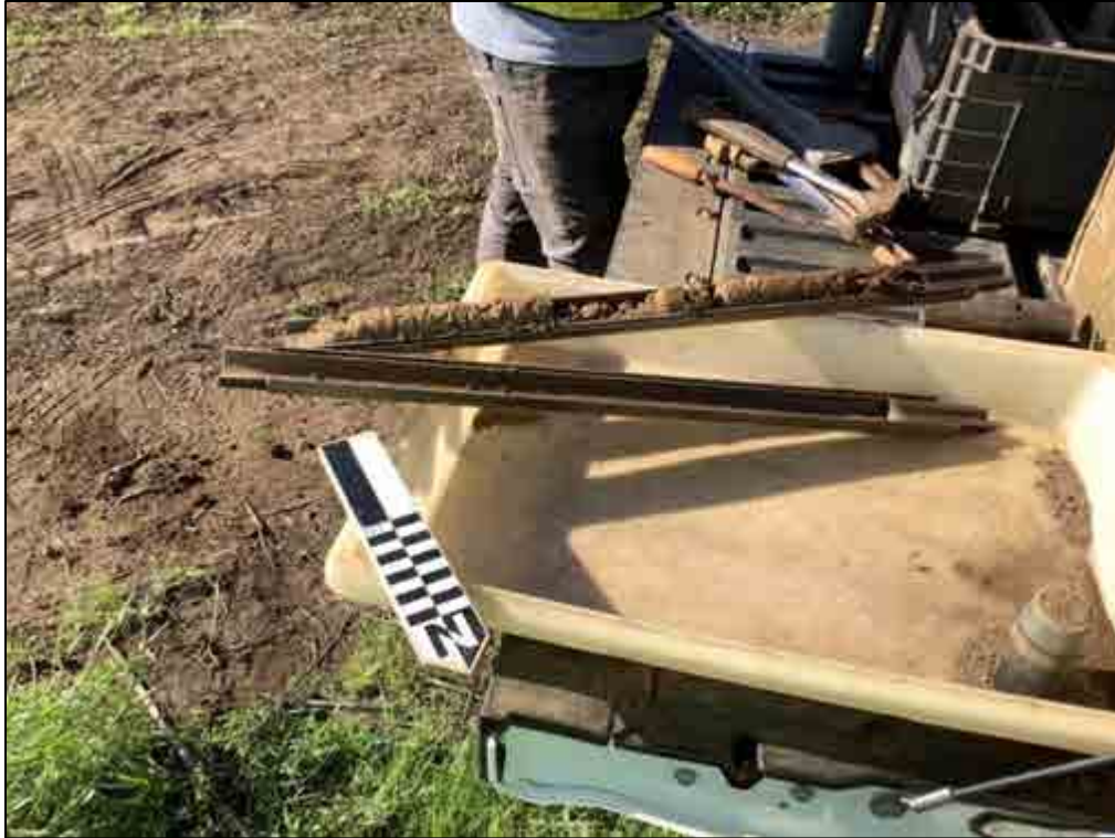
Figure 119. B-27, Sample 3 (1.5-1.9 m), sandy clay loam and silt loam
