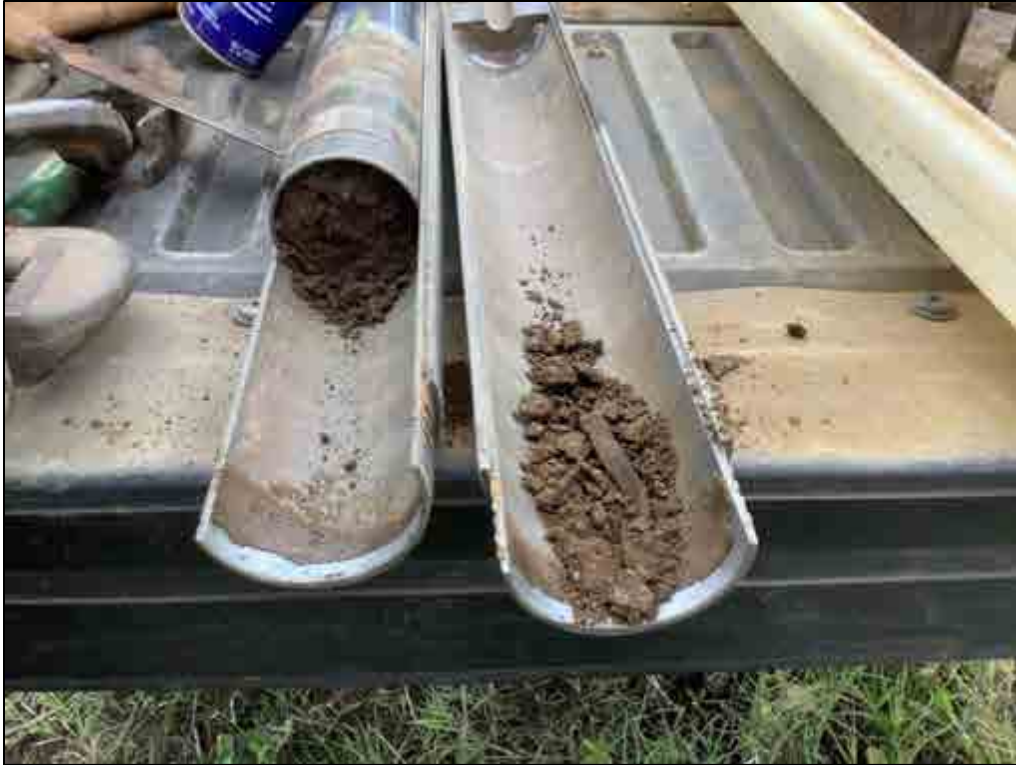
Figure 68. B-1, Sample 1 (0.4-0.9 m), sandy clay loam
