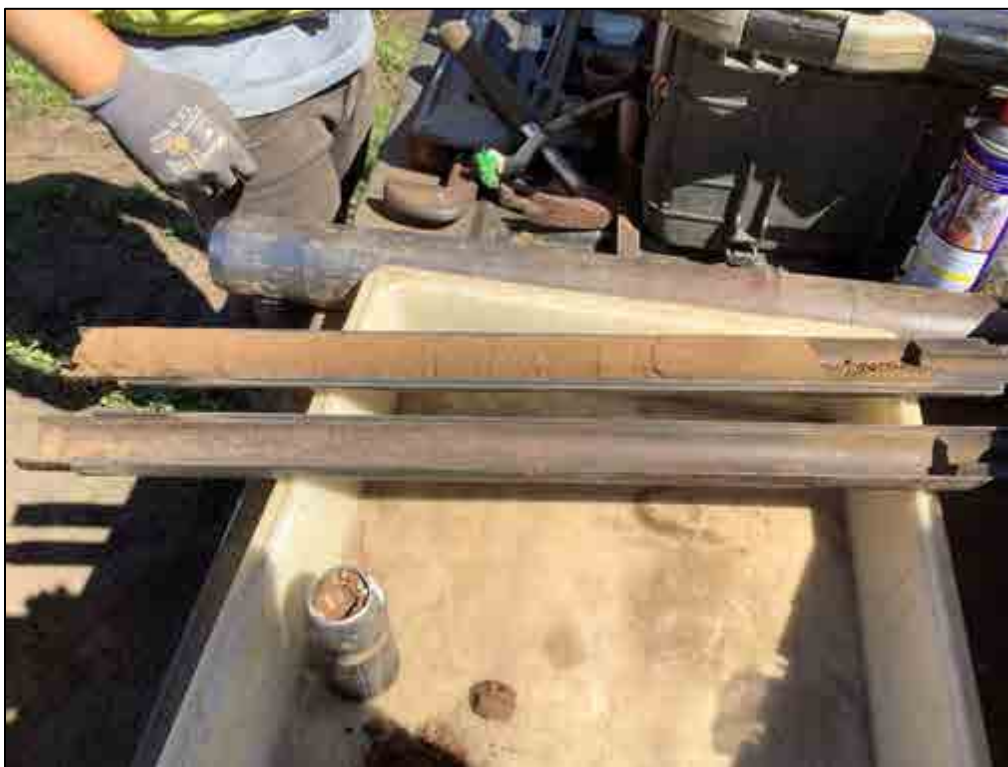
Figure 134. B-34, Sample 4 (2.5-3.0 m), silt loam
