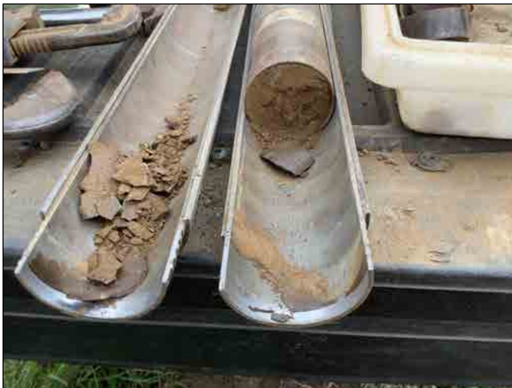
Figure 93. B-13, Sample 4 (0.9-1.5 m), silt loam
