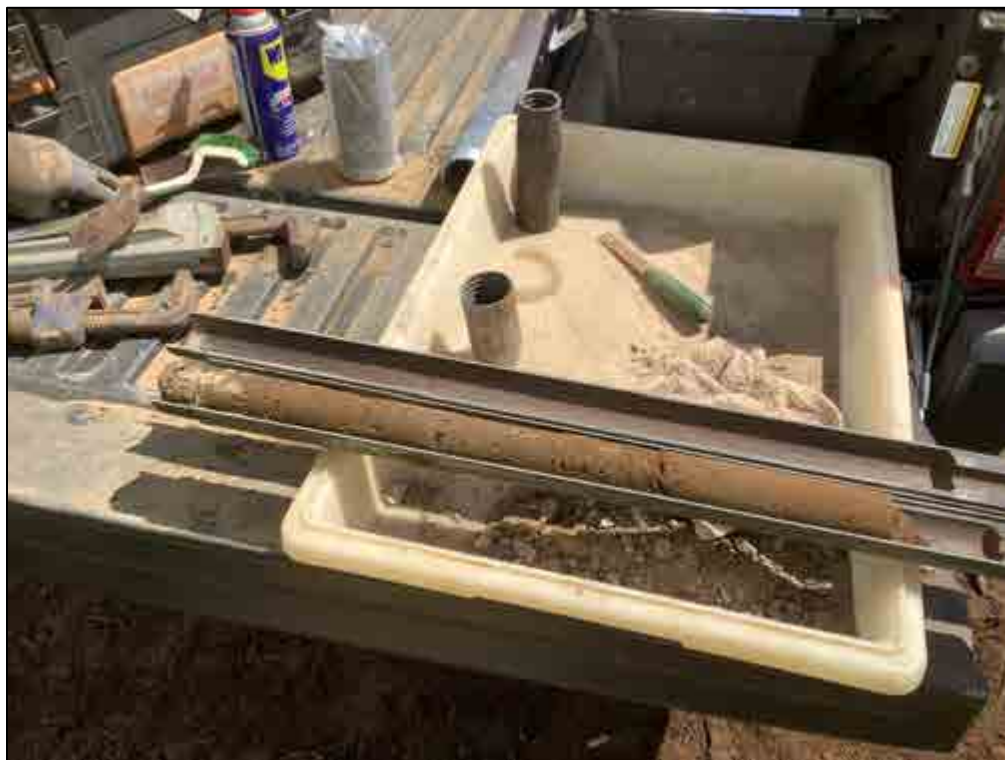
Figure 85. B-9, Sample 5 (4.1-4.5 m), loamy sand and sandy clay loam
