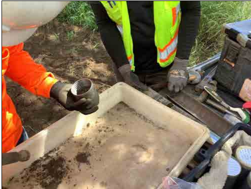
Figure 108. B-21, Sample 1 (0.4-0.9 m), sandy clay loam
