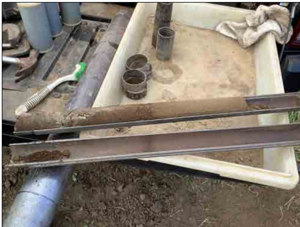
Figure 99. B-16, Sample 5 (4.1-4.5 m) sand and compacted clay loam
