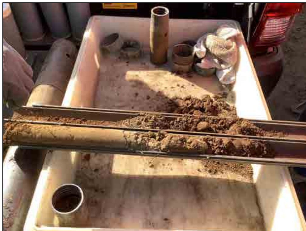
Figure 95. B-14, Sample 4 (2.5-3.0 m), silt loam
