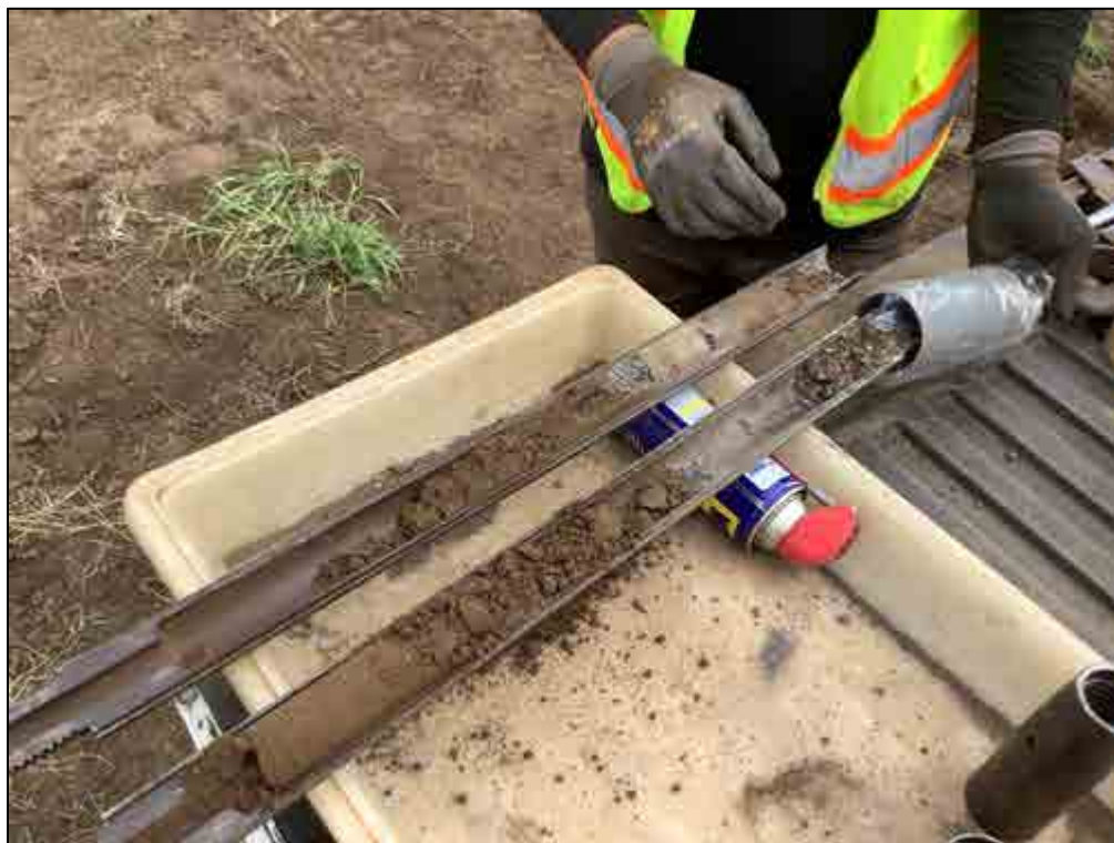
Figure 105. B-19, Sample 6 (5.5-6.0 m), silt loam and gravels
