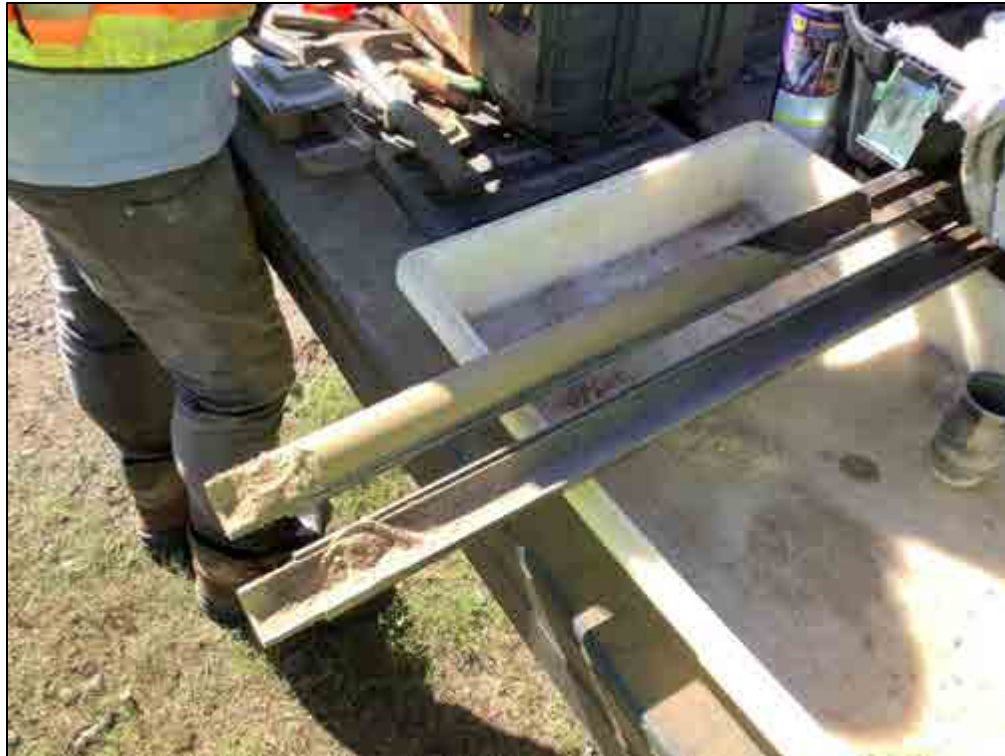
Figure 131. B-33, Sample 4 (4.1-4.5 m), silt loam
