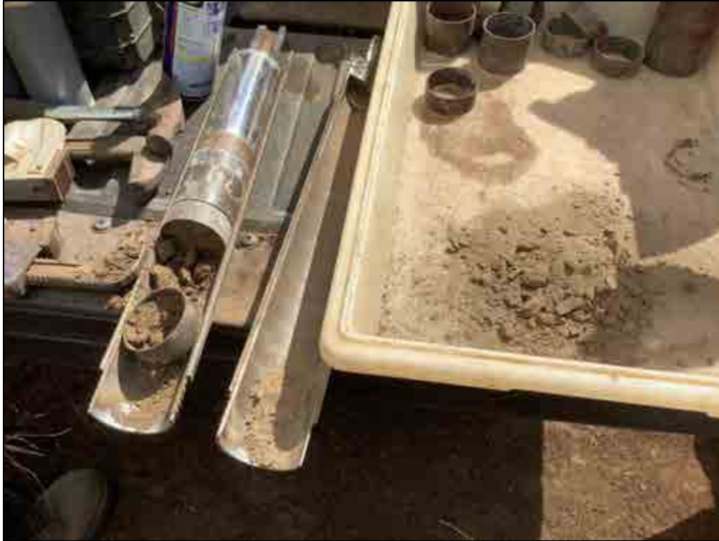
Figure 139. B-37, Sample 3 (1.5-1.9 m), sand
