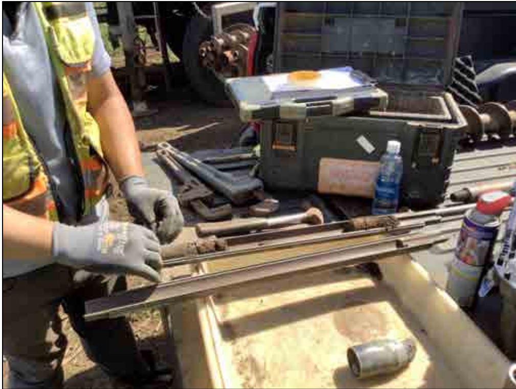
Figure 123. B-29, Sample 2 (0.9-1.5 m), sandy loam and silt loam with gravels
