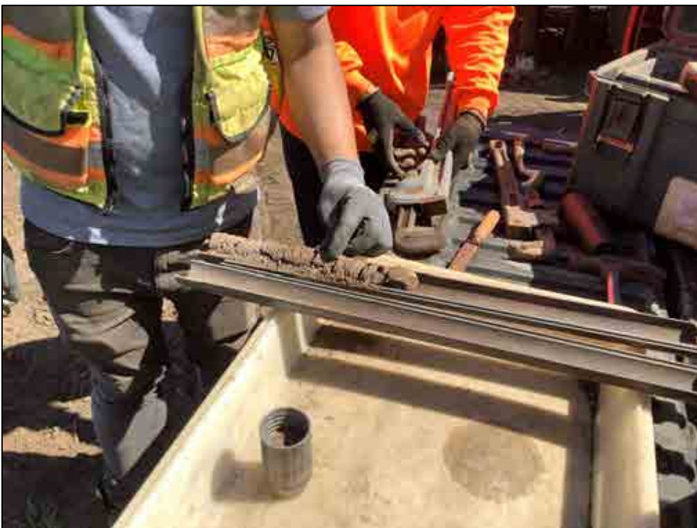
Figure 124. B-29, Sample 4 (2.5-3.0 m), alluvial deposited gravels and silt loam
