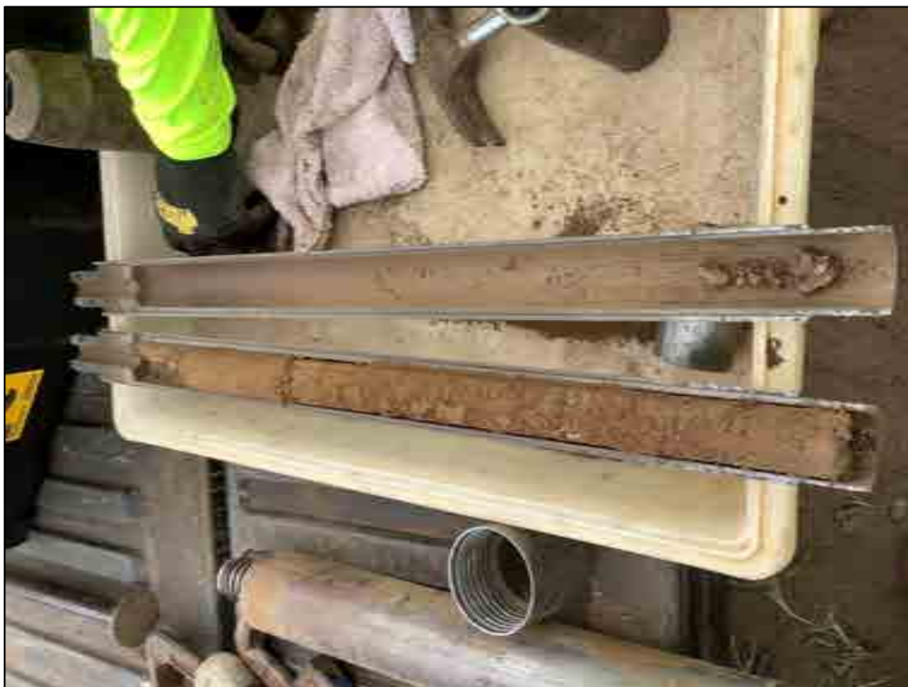
Figure 114. B-24, Sample 5 (4.1-4.5 m), silt loam and gravels
