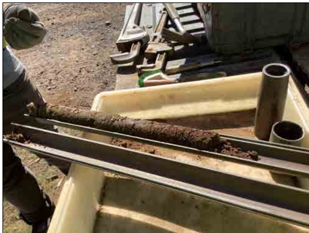
Figure 132. B-33, Sample 6 (5.5-6.0 m), silty clay loam
