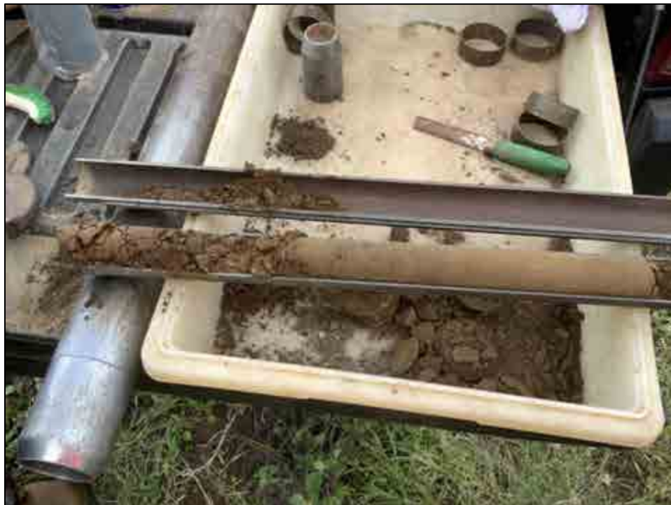
Figure 71. B-2, Sample 4 (2.5-3.0 m), silt loam
