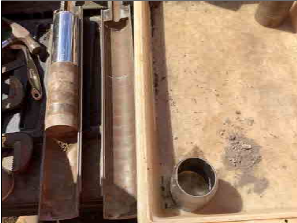
Figure 104. B-19, Sample 2 (0.9-1.5 m), silt loam and gravels
