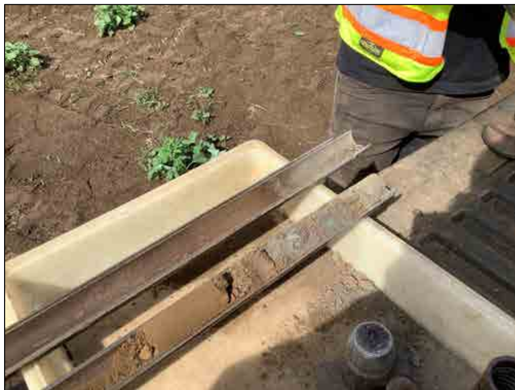
Figure 107. B-20, Sample 5 (4.1-4.5 m), silt loam and loamy sand with gravels
