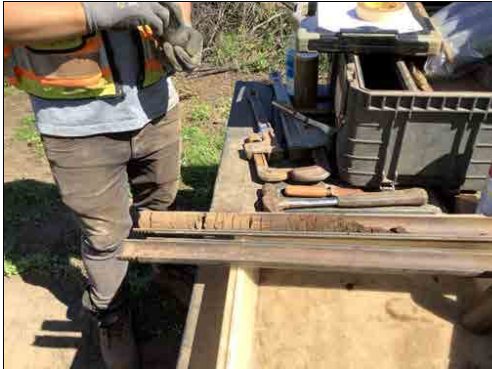
Figure 133. B-34, Sample 2 (0.9-1.5 m), sandy loam and silt loam
