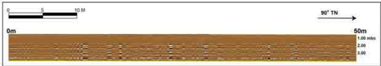
Figure 62. GPR-11 reflection profile (0-50 m)
