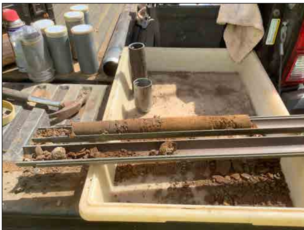
Figure 83. B-8, Sample 6 (5.5-6.0 m), silt loam, silty clay loam, and alluvial deposited gravels
