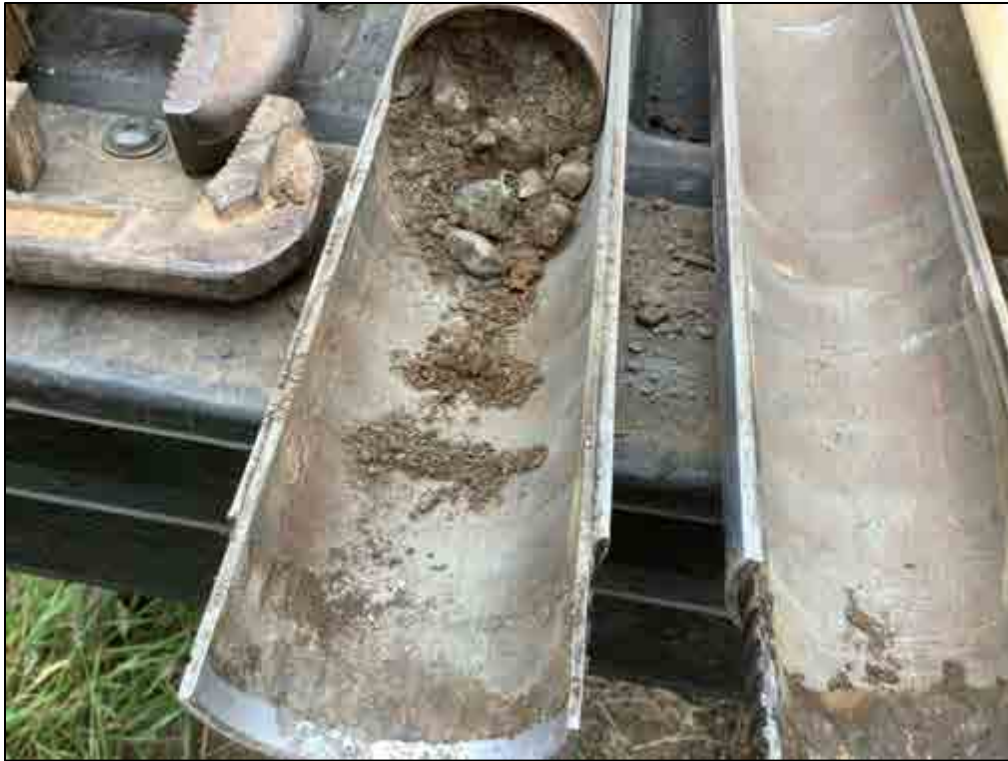
Figure 92. B-13, Sample 2 (0.9-1.5 m), loamy sand and gravels
