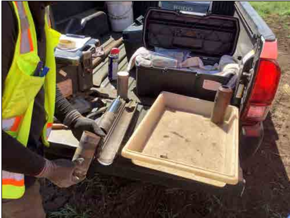
Figure 102. B-18, Sample 2 (0.9-1.5 m), silty clay loam
