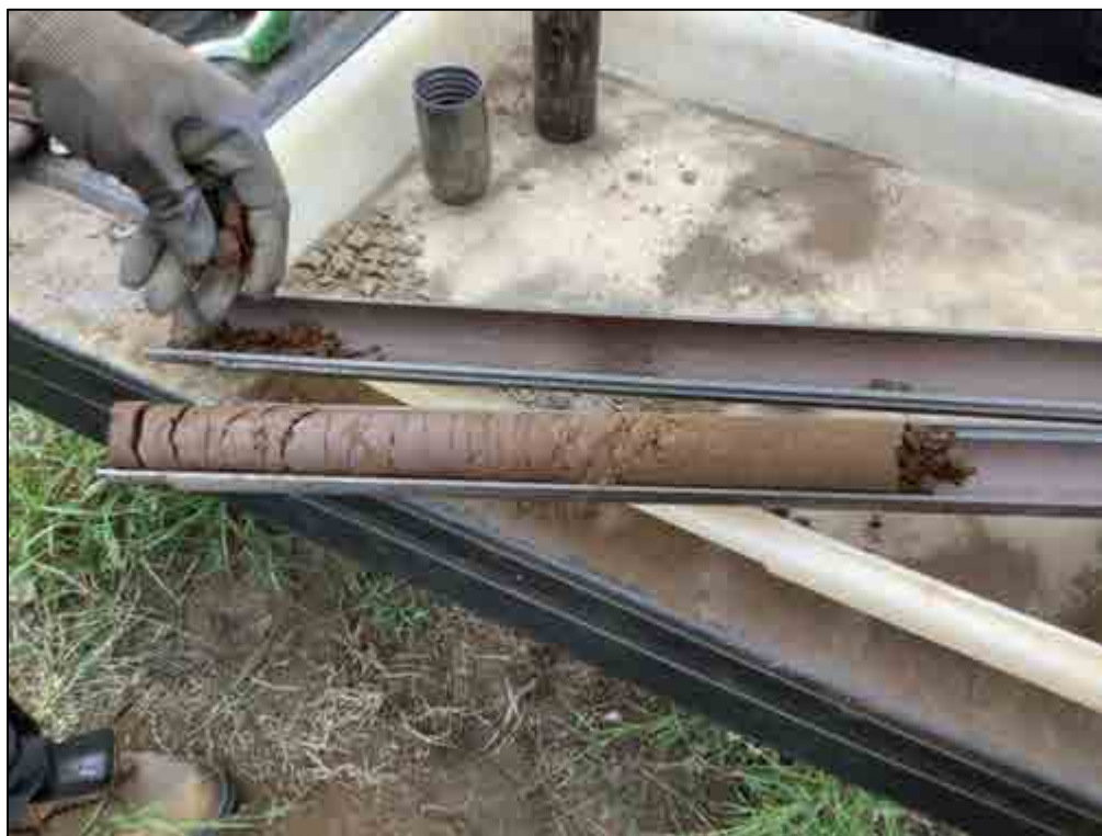
Figure 73. B-3, Sample 6 (5.5-6.0 m), silt loam and silty clay loam
