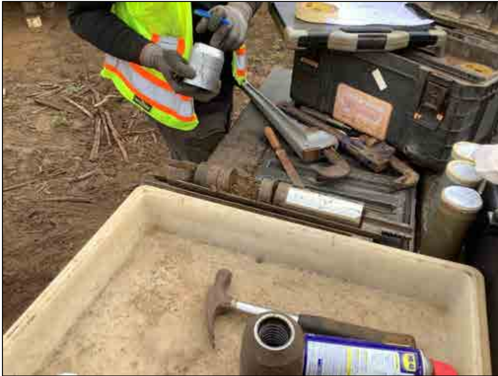
Figure 110. B-22, Sample 3 (1.5-1.9 m), silt loam
