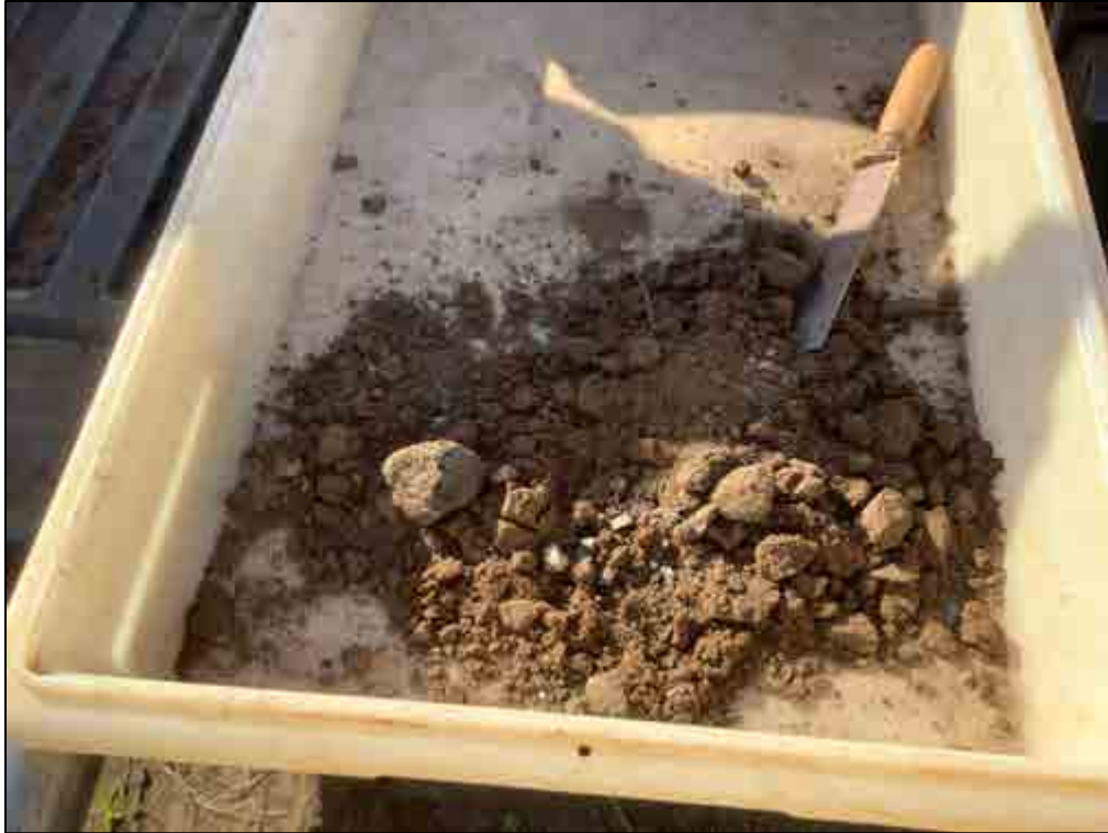
Figure 90. B-12, Sample 1 (0.4-0.9 m), sandy loam and gravel
