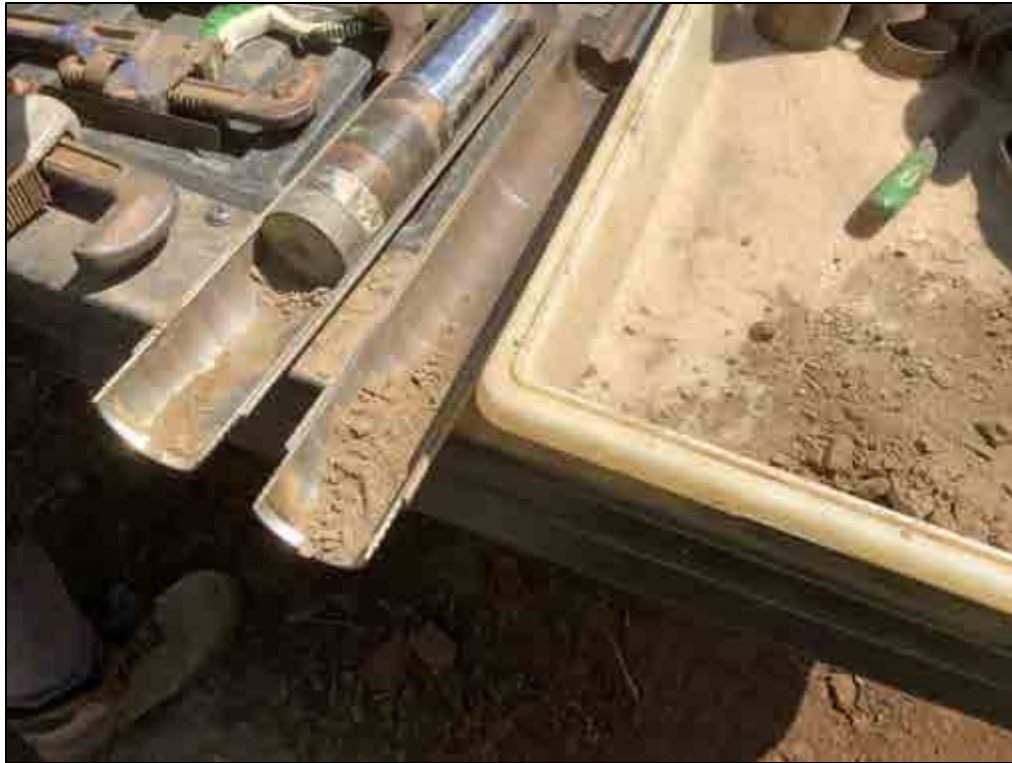
Figure 84. B-9, Sample 3 (1.5-1.9 m), silt loam
