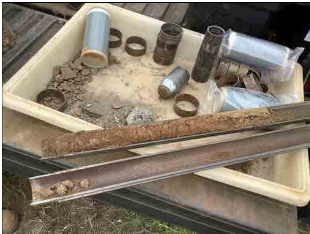
Figure 77. B-5, Sample 3 (1.5-1.9 m), silt loam
