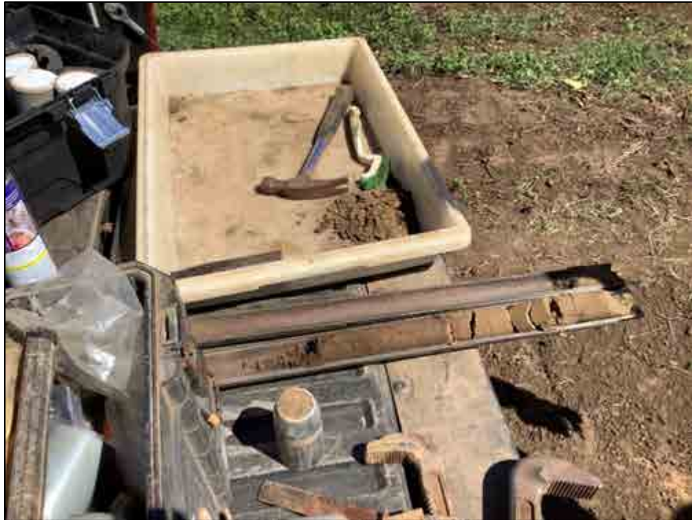
Figure 135. B-35, Sample 2 (0.9-1.5 m), sandy loam and loamy sand
