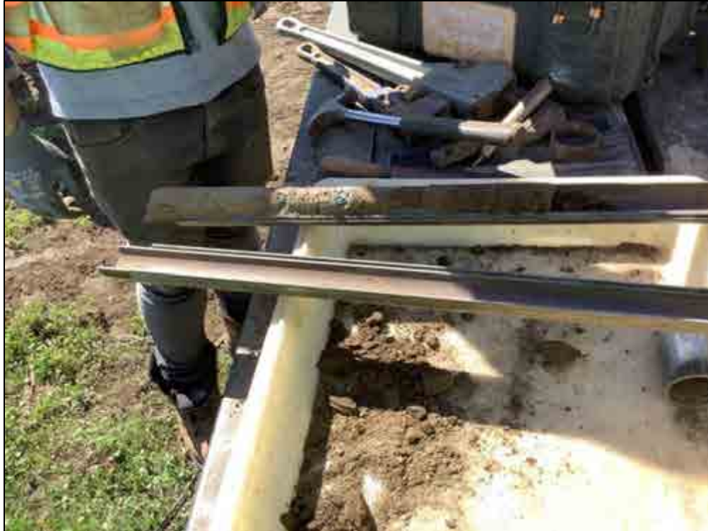
Figure 137. B-36, Sample 3 (1.5-1.9 m), sandy loam and silt loam
