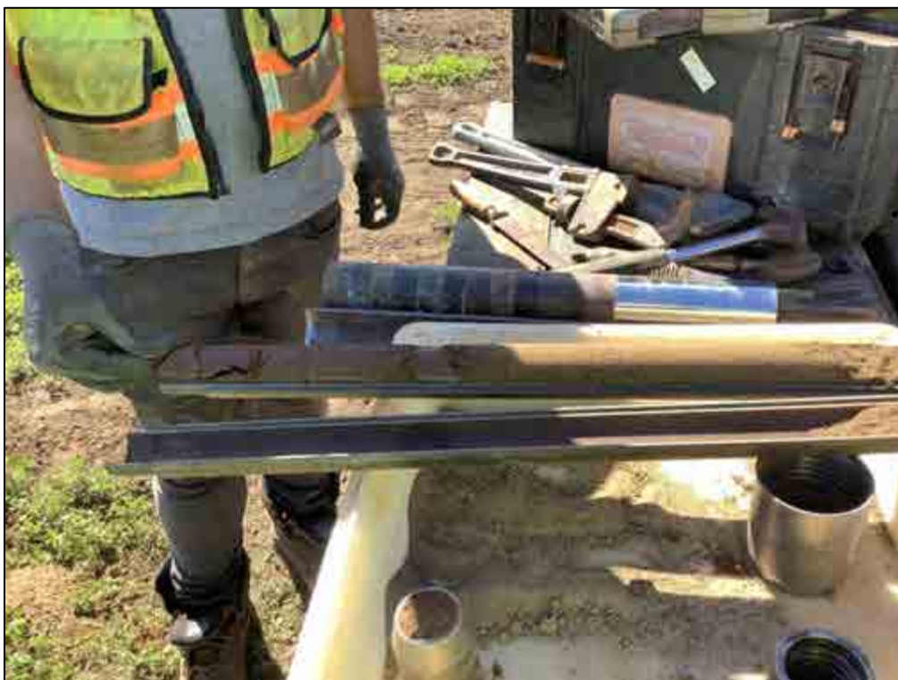
Figure 138. B-36, Sample 6 (5.5-6.0 m), sand and silty clay loam
