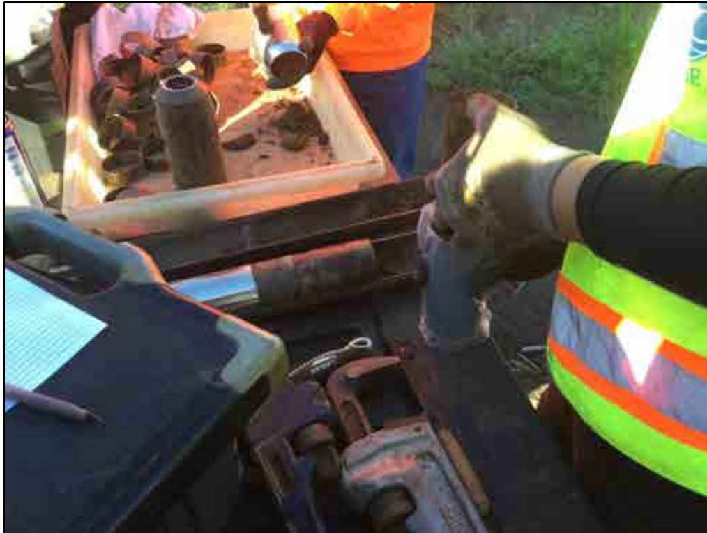
Figure 78. B-6, Sample 2 (0.9-1.5 m), collection methods
