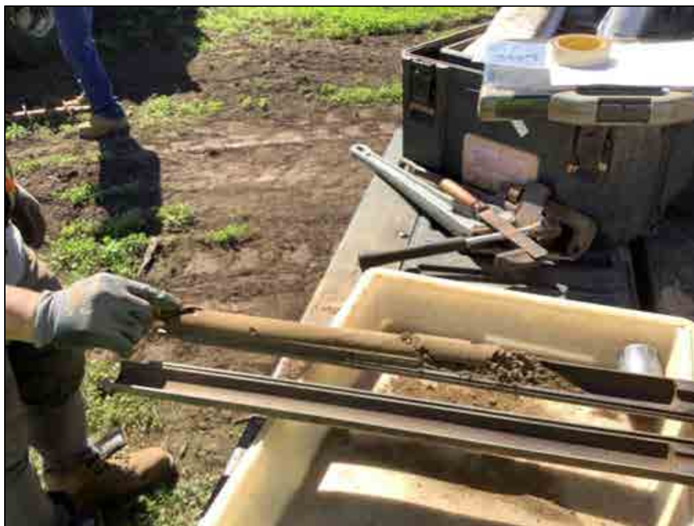
Figure 118. B-26, Sample 3 (1.5-1.9 m), sand and silt loam
