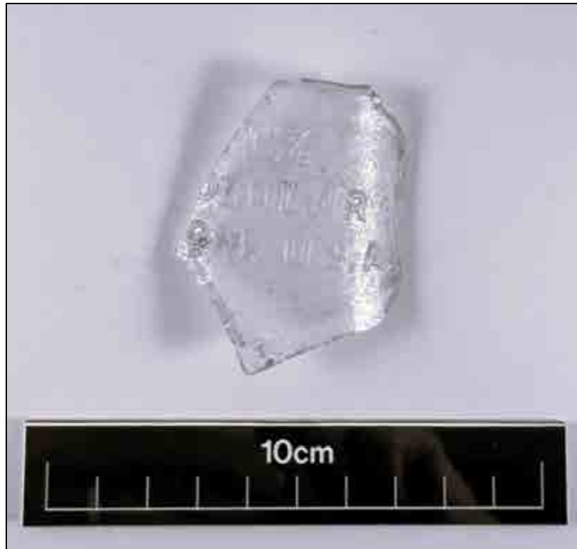
Figure 173. Accession # 94, embossed glass, a glass lantern cover from R.E. Dietz Company, New York City, USA est. 1840
