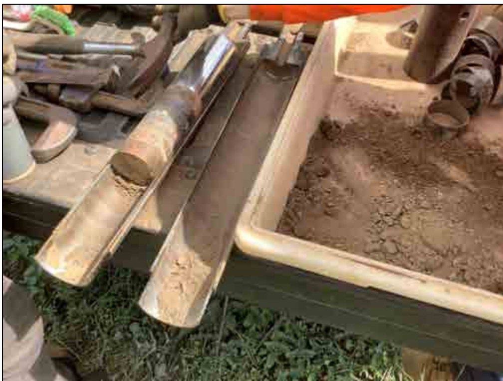
Figure 101. B-17, Sample 3 (1.5-1.9 m), silt loam
