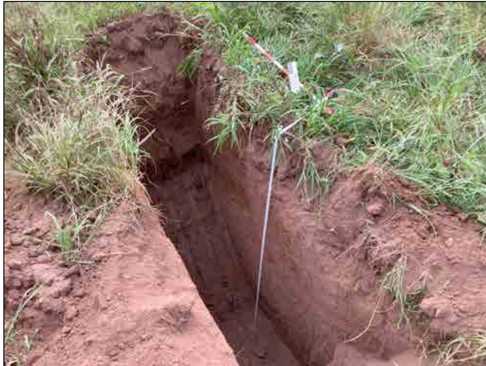
Figure 159. TP-17 observed stratigraphy (0.0-2.2 m), view to south
