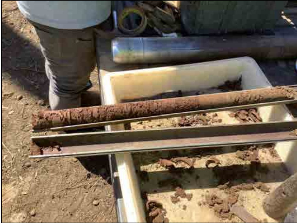
Figure 127. B-31, Sample 4 (4.1-4.5 m), silt loam and silty clay loam
