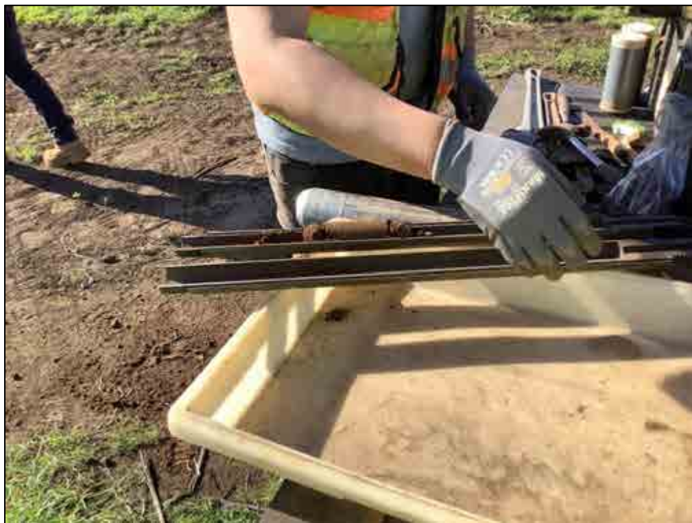
Figure 120. B-27, Sample 5 (4.1-4.5 m), silty clay loam
