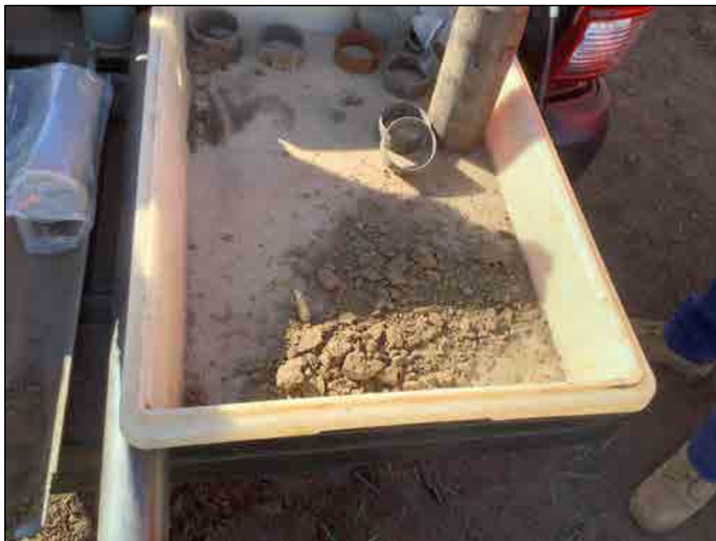
Figure 91. B-12, Sample 3 (1.5-1.9 m), silt loam
