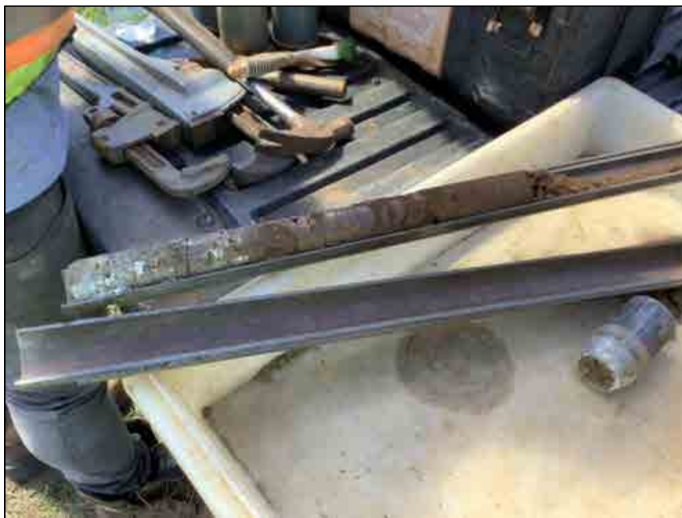
Figure 122. B-28, Sample 4 (2.5-3.0 m), sandy loam and silty clay loam with gravels
