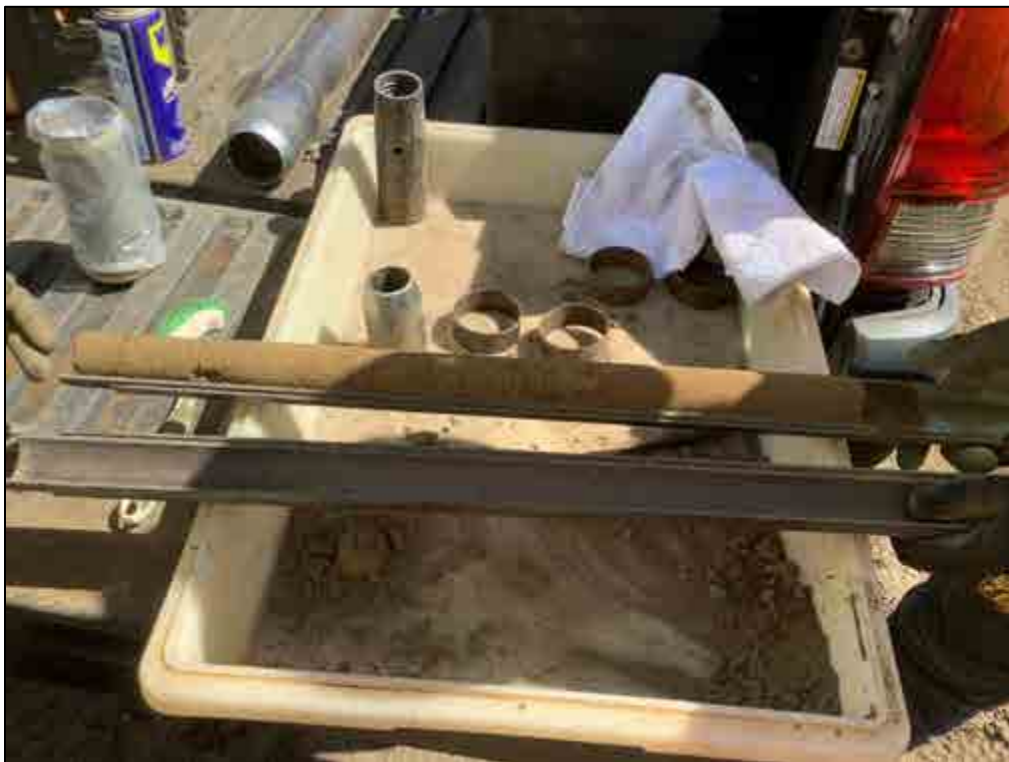
Figure 75. B-4, Sample 5 (4.1-4.5 m), silt loam
