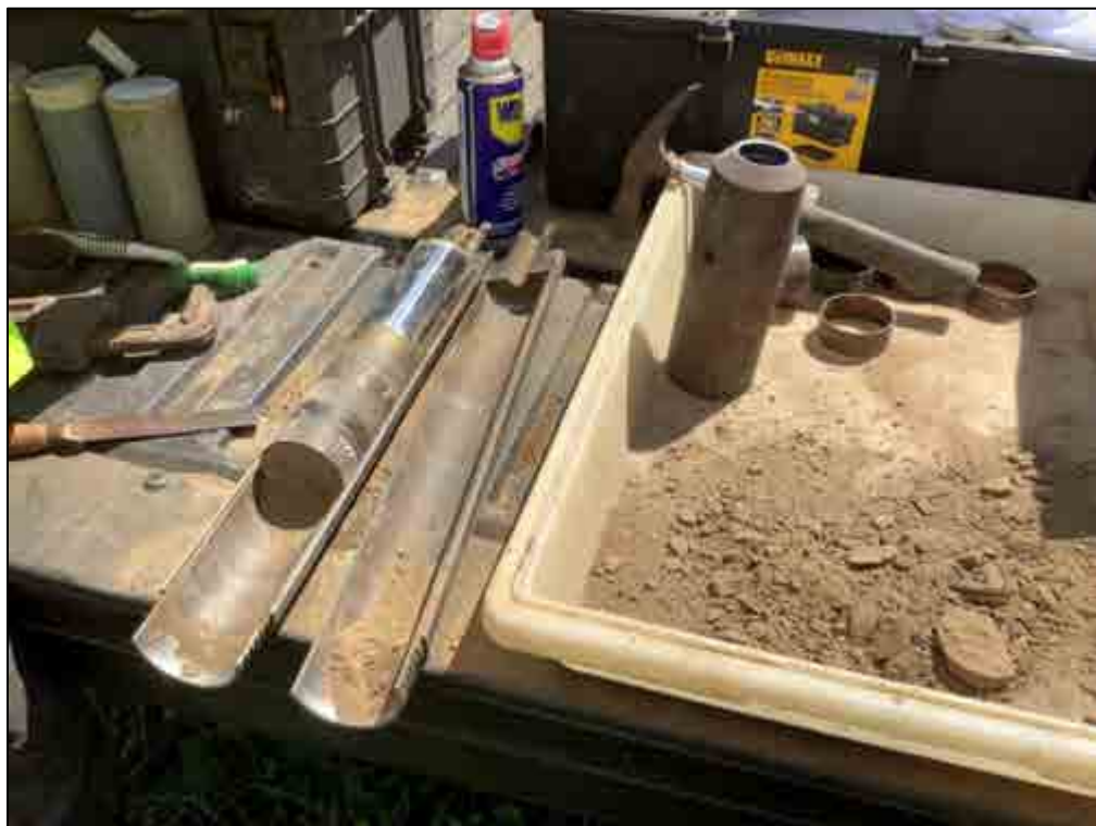
Figure 142. B-38, Sample 4 (2.5-3.0 m), sand
