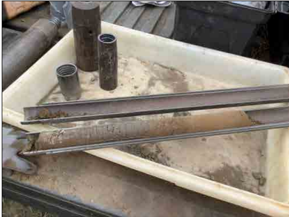
Figure 72. B-3, Sample 3 (1.5-1.9 m), silt loam and silty clay loam
