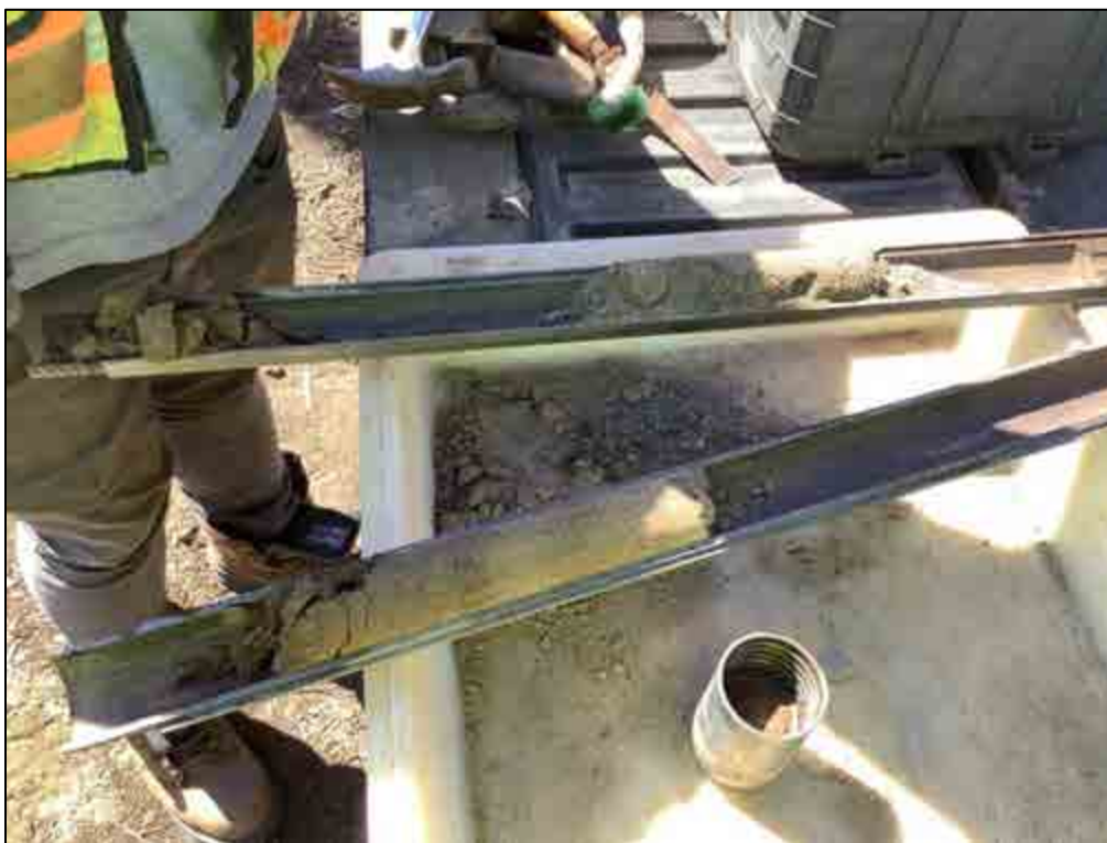
Figure 136. B-35, Sample 4 (2.5-3.0 m), sand and silt loam
