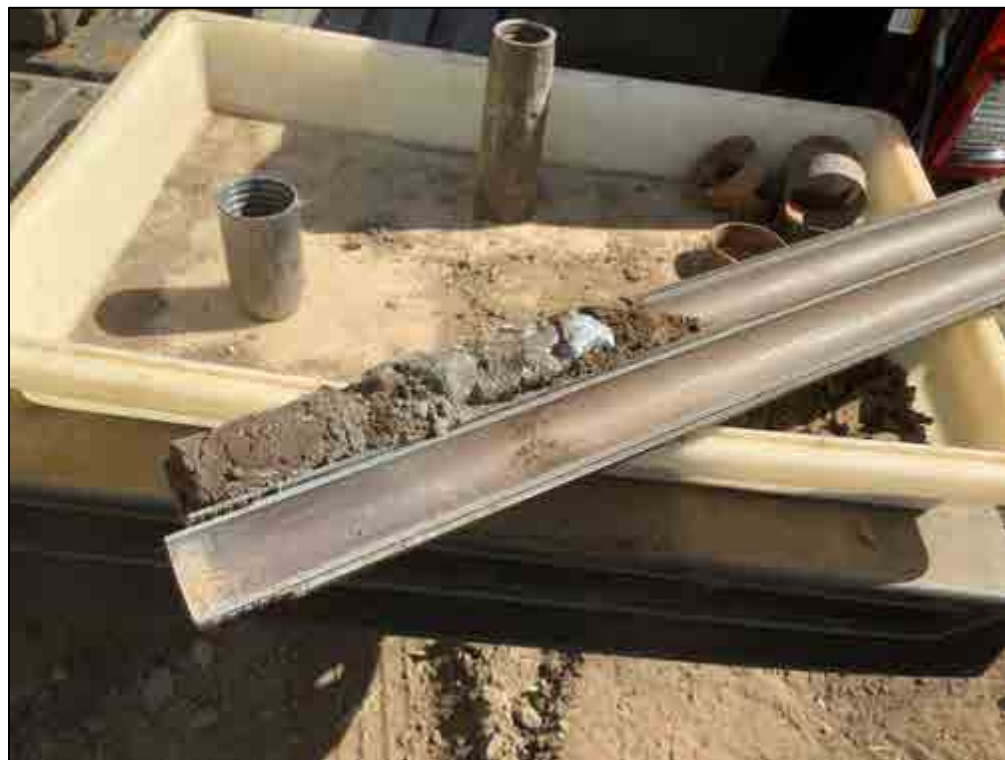
Figure 81. B-7, Sample 5 (4.1-4.5 m), alluvial loamy sand and gravel
