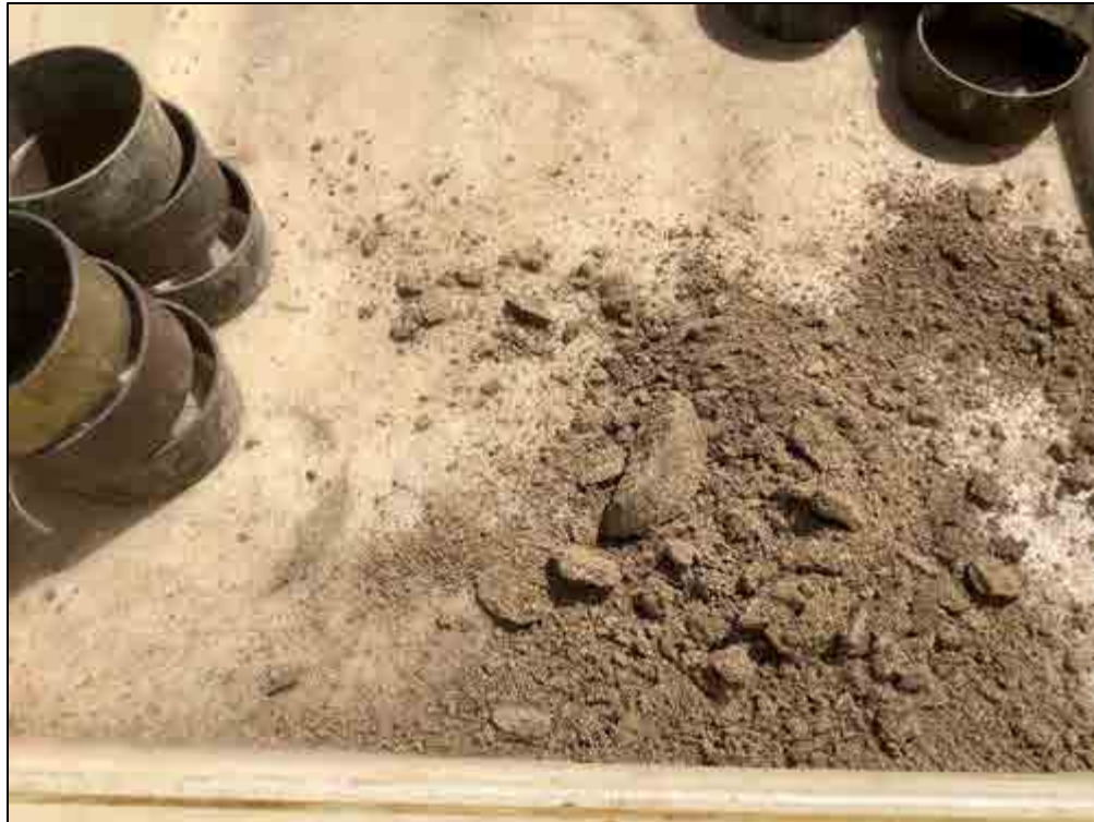
Figure 117. B-26, Sample 2 (0.9-1.5 m), loamy sand
