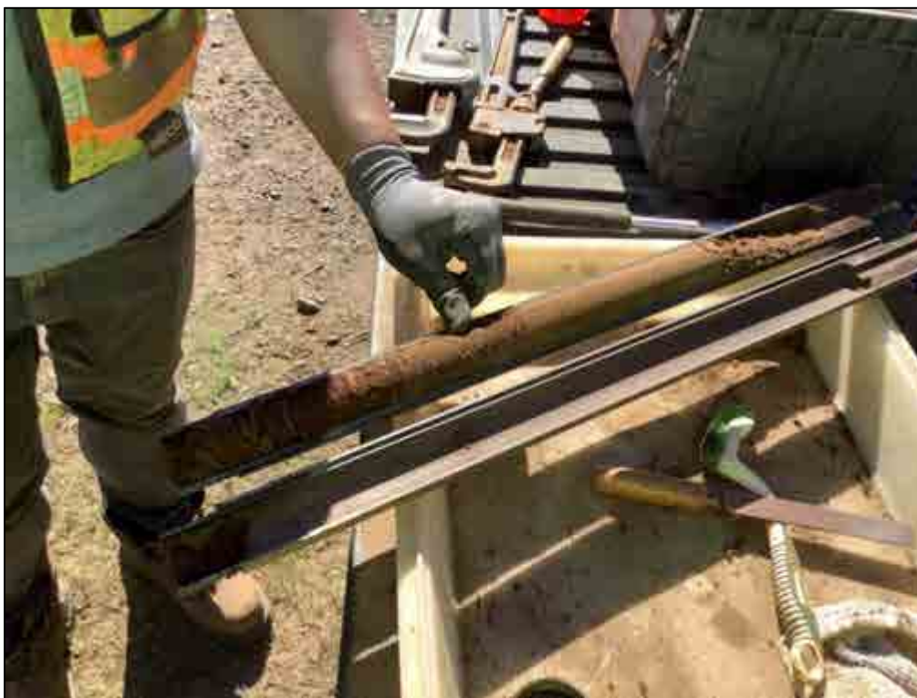
Figure 126. B-30, Sample 5 (4.1-4.5 m), loamy sand and silty clay loam
